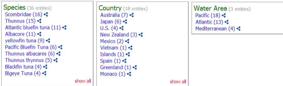
Fig. 5. The result of entity mining (configured to identify fish species, countries and water areas) for the query tuna species
