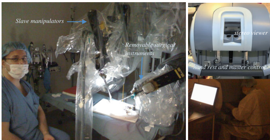
Fig. 3 The da Vinci surgical system (Intuitive Surgical, Inc.): a first-generation slave (patient-side manipulators) setup for a training session ( left ), and a second-generation master console ( right, top ) and the system in use by a trainee surgeon and bottom. Until the introduction of near infrared fluorescence integration recently, only visual imaging was available for feedback to the surgeon. Any additional imaging was viewable as a video ( picture in picture ) piped from external consoles ( right bottom ). A new version of the da Vinci system—the da Vinci Xi—has been introduced in 2014 that significantly improves positioning of the surgical instruments over the patient and reduces the operating room footprint
