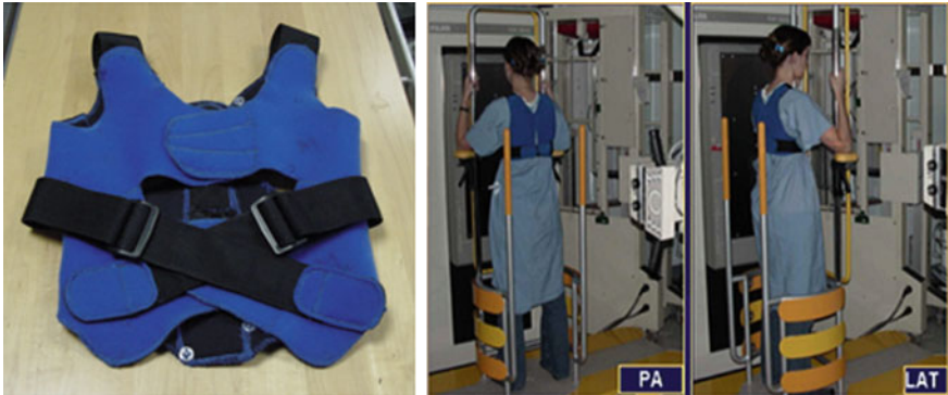
Fig. 3 Left Calibration vest worn by the patient and the positioning system used at the Sainte-Justine Hospital. The calibration vest has embedded radio-opaque markers visible on the biplanar to self-calibrate the scene using fiducial points closer to the patient's skin. Right Positioning system to minimize patient motion between biplanar acquisitions
