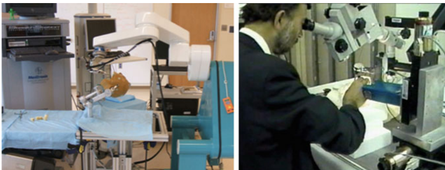
Fig. 2 Examples of research systems: a NEUROMATE (Integrated Surgical Systems, Inc.) neurosurgical experimental setup at the Johns Hopkins University ( left ), and a user manipulating the first generation “steady-hand” surgeon’s assistant microsurgery system ( right )
