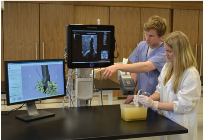
Fig. 11 A simulator with tracked ultrasound, tracked needle, and registered 3-D anatomical model for learning spatial coordination in spinal interventions
