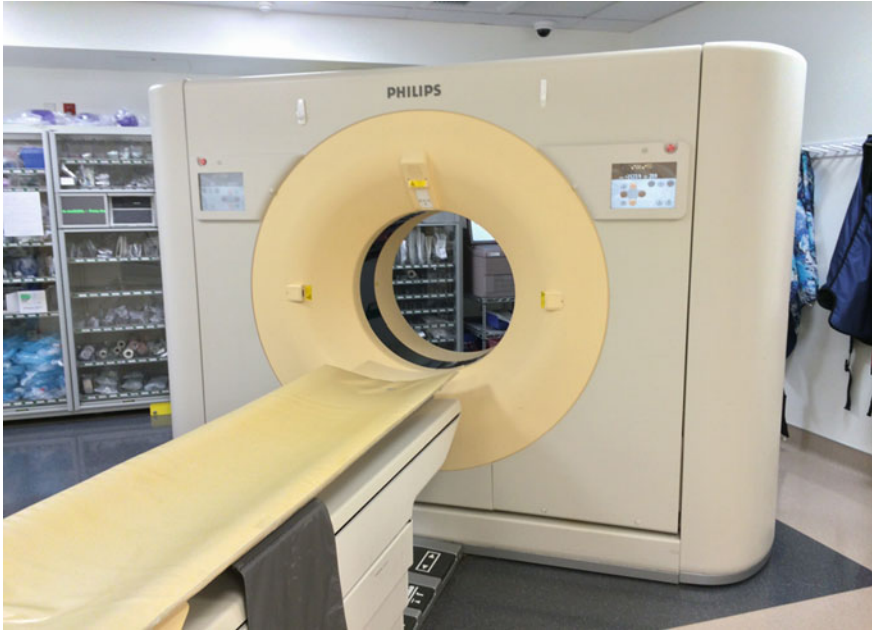
Fig. 4 Typical CT scanner unit. Patient is placed in alignment with the central axis of the helical trajectory traced by the X-ray beam source and detectors as they rotate about the patient
