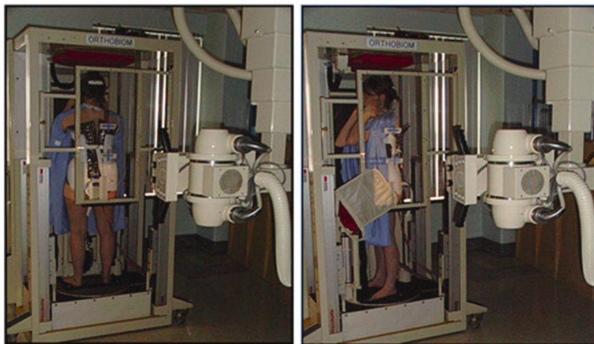
Fig. 2 One of the first 3D reconstruction systems installed at the Sainte-Justine Hospital in 1992, where a plexiglass cage with embedded pellets is used to calibrate the X-ray scene. The patient is turned from the frontal to sagittal position to obtain biplanar radiographs
