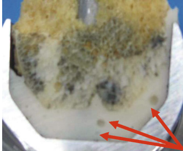
Fig. 10 Macroscopic view of a failed hip prosthesis, showing the trapped air bubble into the cement mantle
