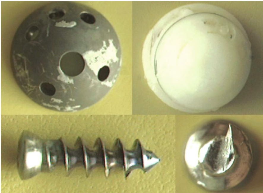
Fig. 4 Macroscopy view of the primary implant components that were analyzed: acetabular cup, polyethylene liner, screws
