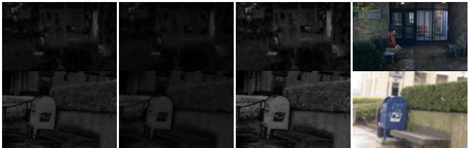
Fig. 5. Raindrops/Snowflakes removal results with guided image filtering: first row shows removal result for sitting man in rain weather; second row shows removal result for mailbox in snow weather. From left to right: I_f , I_{mean} , I_{guidance} and weather removal result.
