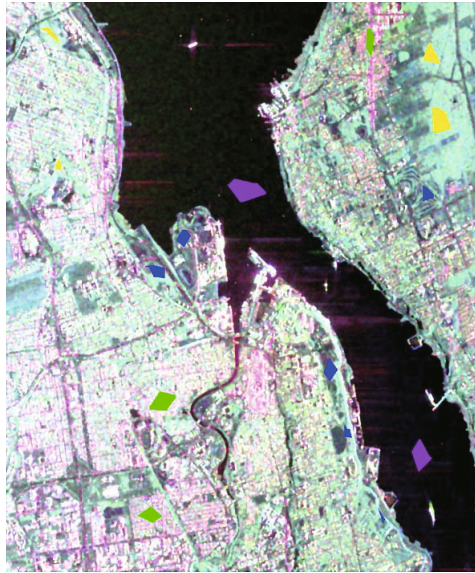
Fig. 1. The false color composite image with learning samples based on Pauli matrix factorization
