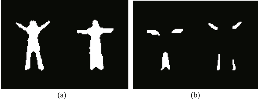
Fig. 1. DS between two adjacent silhouettes. (a) The silhouette of different frames. (b) Forward difference silhouette and backward difference silhouette extracted from (a).
