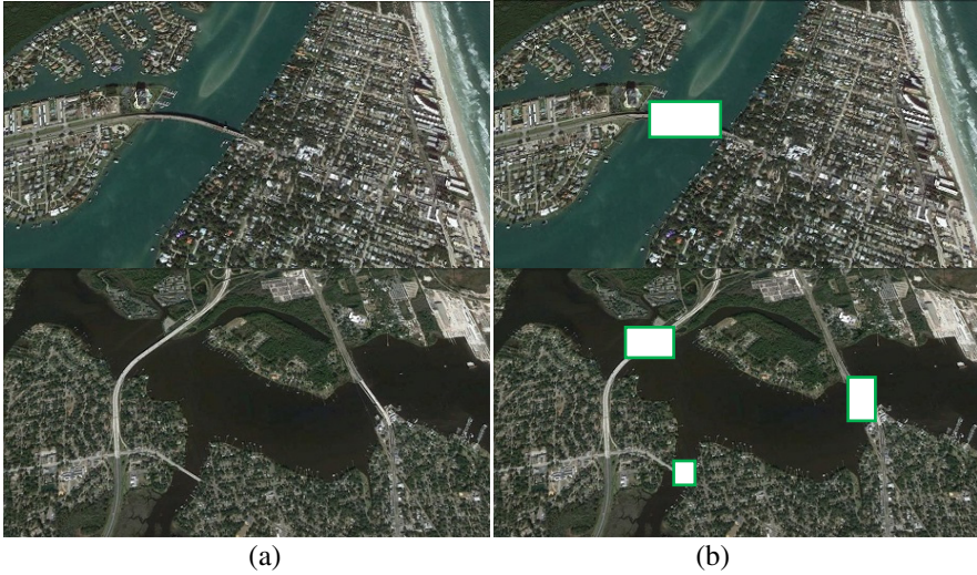
Fig. 1. Bridge detection in panchromatic imagery with our proposed algorithm: (a) represents the original satellite data; (b) demonstrates bridge detection results
