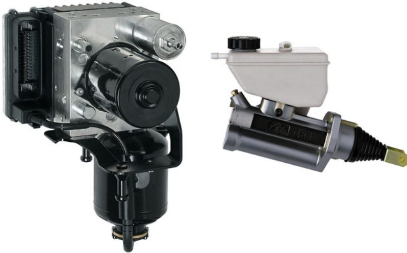
Fig. 13 EHB components by Continental ( left , electrohydraulic control unit; right , brake actuator with pedal characteristic simulator)
