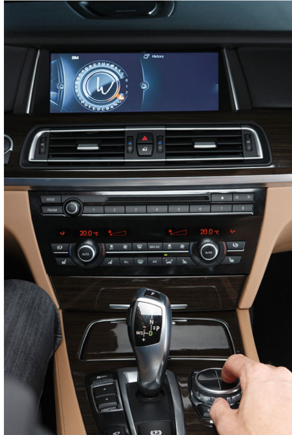
Fig. 5 Menu system with display and central control element: BMW iDrive (Source: BMW AG)
