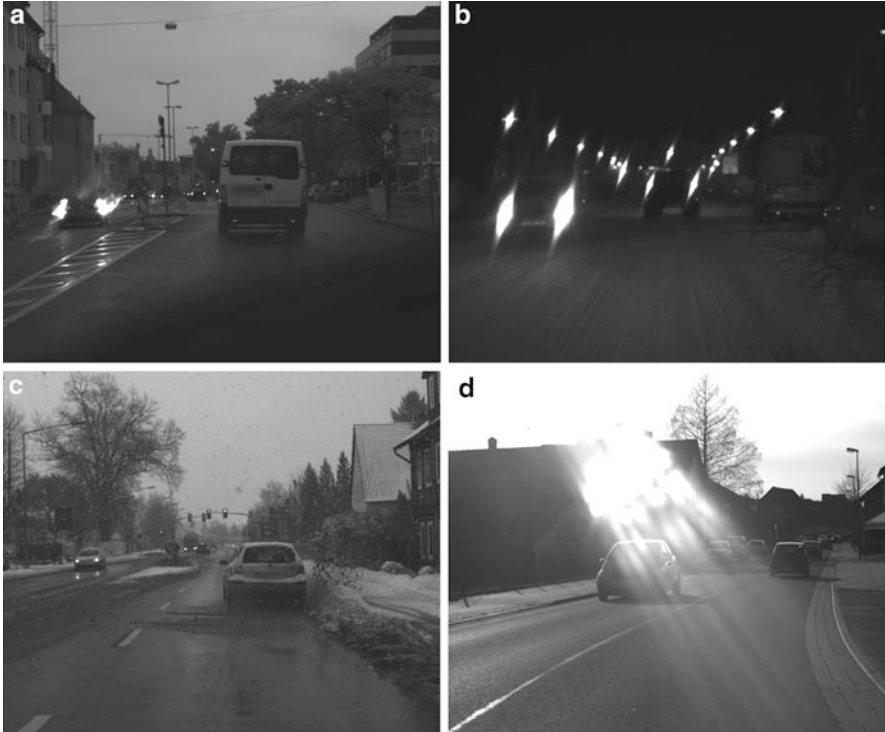
Fig. 1 Safety-critical driver assistance applications pose high demands on the robustness of algorithms. (a) When raining, blinding and windshield smear can occur due to water on the windshield. (b) At nighttime, windshield wipers can generate disturbances with characteristic smear artifacts. (c) Snow fall and wet streets cause problems in disparity estimation. (d) Backlight can generate reflections on the windscreen that must not lead to erroneous obstacle detection (Figures courtesy of the HCI benchmark of D. Kondermann, University of Heidelberg (Meister et al. 2012))
