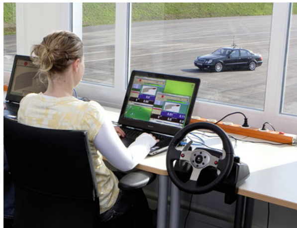
Fig. 3 Remote control of automated vehicles from control station
