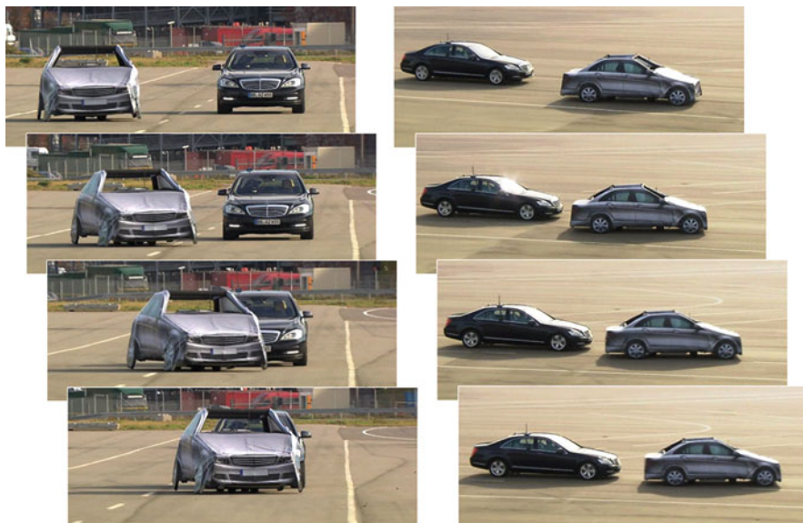
Fig. 8 Cut-in maneuver with coordinated vehicle and target
