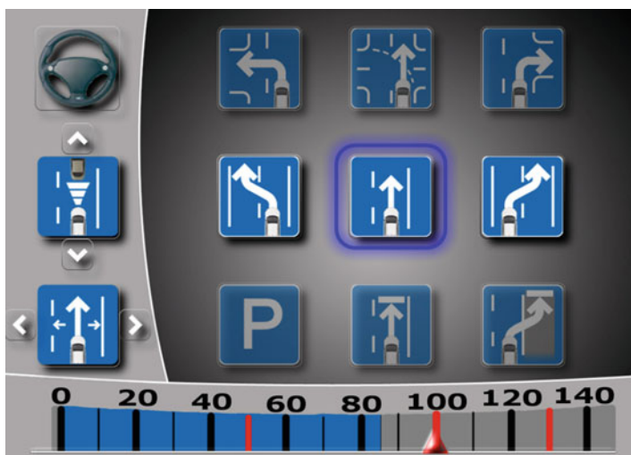
Fig. 7 Content depicted on the tactile touch display (From Franz et al. (2011), derived from Kauer et al. (2010)). In this example, the maneuver “lane change left/right” is available, and the maneuver “follow the course of the road” is active. Desired speed is set to 100 km/h, while the vehicle is currently driving at about 85 km/h
