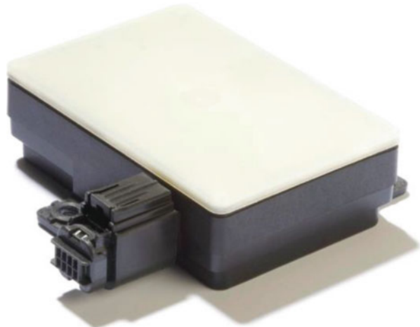
Fig. 51 External view of the Valeo MBH RADAR (Source: Valeo)
