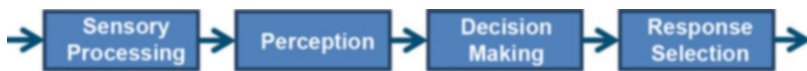
Fig. 2 Simple information processing system (Based on Luczak (1975). Representation from Parasuraman et al. (2000))
