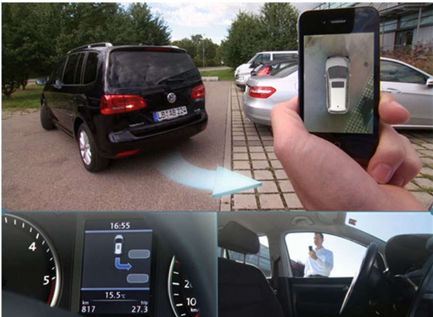
Fig. 15 Remote parking – level 2 automatization
