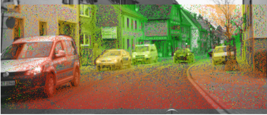
Fig. 2 Color-coded disparity image ( red nearby . . . green far) overlaid on the original image. The disparity image does not contain a result for every pixel (no color overlay). Isolated outliers ( red points in the background) are visible
