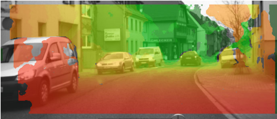
Fig. 4 Two color-coded disparity image ( red nearby ... green far) obtained by GraphCut overlaid on the original image. A visually error-free disparity image is generated. However, computation time exceeds 10 s (in 2014)
