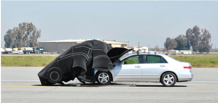
Fig. 10 Propulsion and target system “guided soft-crash target” by company Anthony Best Dynamics, UK (ABD 2014)
