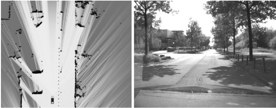
Fig. 13 Grid map of an actual vehicle environment
