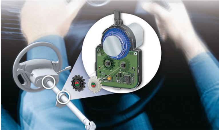
Fig. 5 Possible installation position of steering angle sensor
