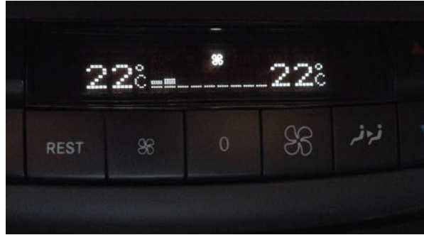
Fig. 13 OLED display in the Mercedes E-Class (2005) for climate control
