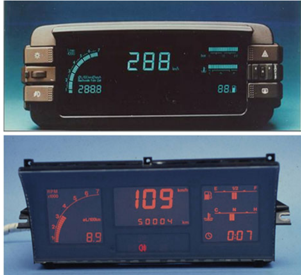
Fig. 3 Digital instrument cluster of the Audi Quattro in VFD technology ( top ) and in LCD technology ( bottom )
