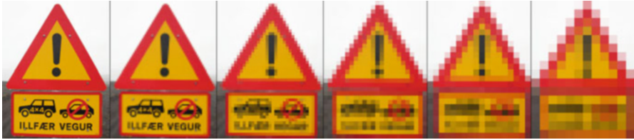
Fig. 6 Effect of decreasing resolution using the example of a traffic sign ( 480 \times 650/72 \times 96/36 \times 48/24 \times 32/18 \times 24/12 \times 16 )
