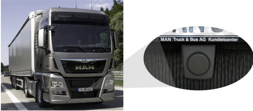
Fig. 5 Installation situation of an ACC sensor on the truck
