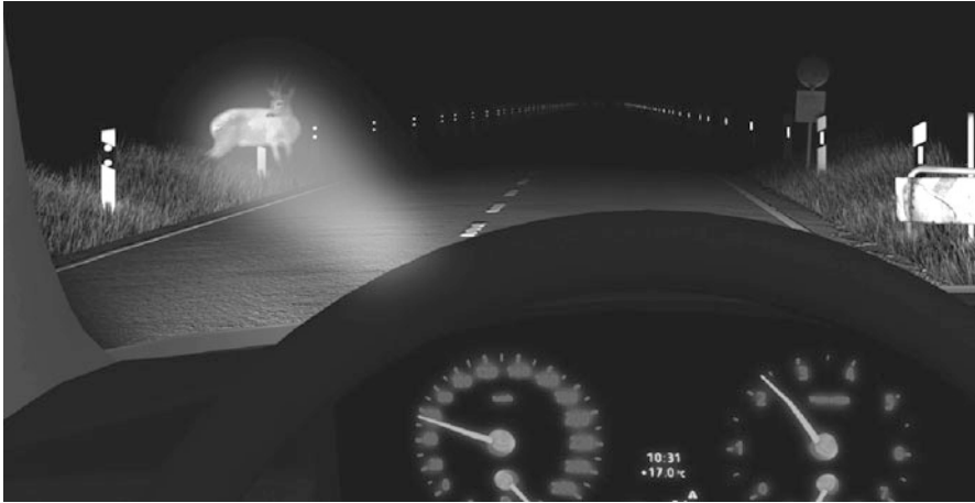
Fig. 19 Principle of marking light (Image source: Hella (Kleinkes et al. 2007))
