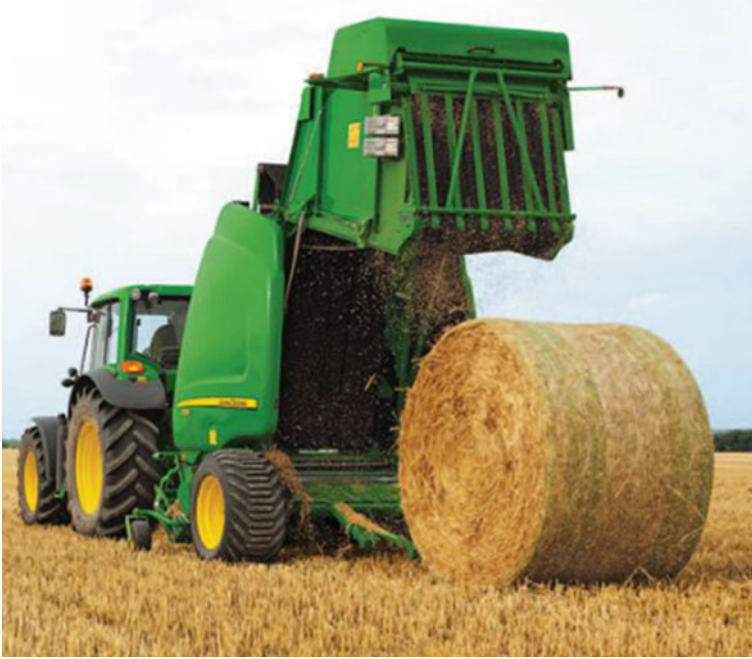
Fig. 8 Tractor with roundbaler ejecting a bale
