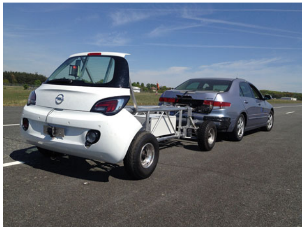
Fig. 1 EVITA (consisting of towing vehicle and dummy target)
