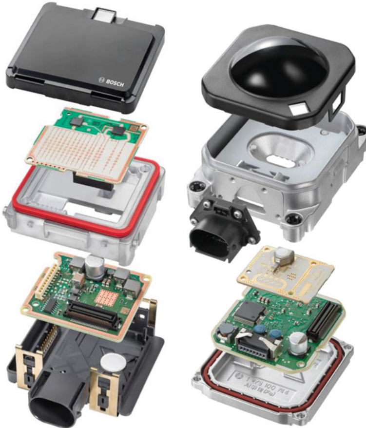
Fig. 30 Construction of the Bosch RADAR sensors MRR and LRR3 (Source: Bosch)
