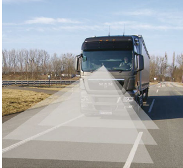
Fig. 7 Installation situation for a camera in a truck for detection of lane markings [Source: MAN Truck & Bus AG]
