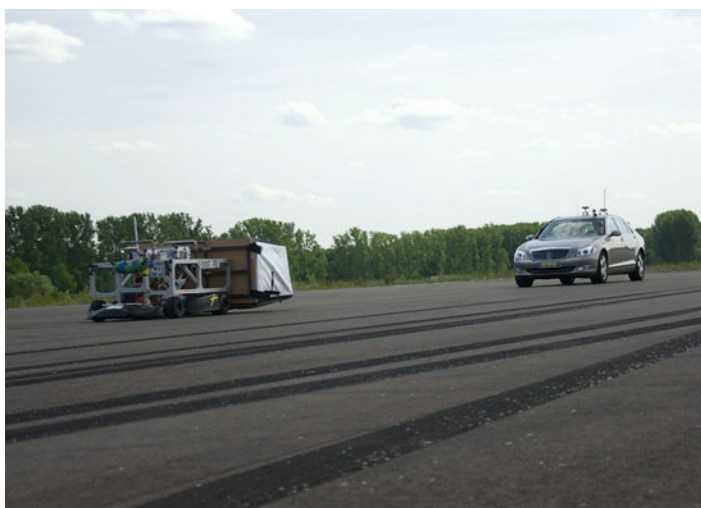
Fig. 4 Driving tests with a first prototype of the ASSESSOR and BAST's propulsion system
