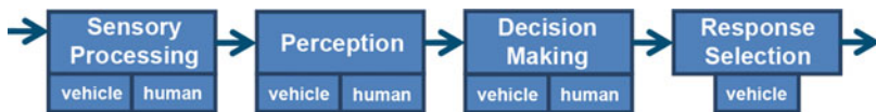
Fig. 3 Fundamental division of tasks in Conduct-by-Wire based on simple information processing systems as outlined by Luczak (1975) (Representation from Franz (2014))
