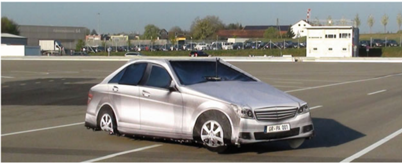
Fig. 4 Concept of the self-driving soft crash target
