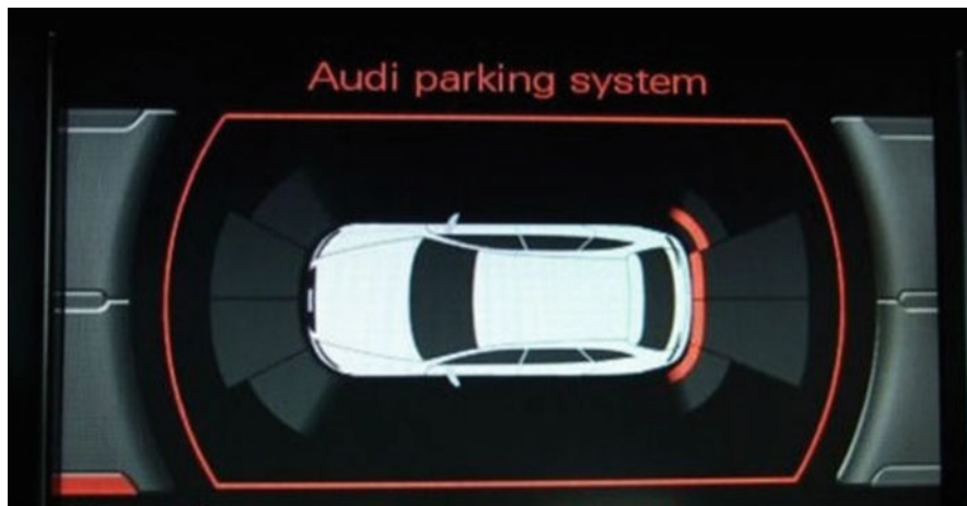
Fig. 6 Example of parking aid in an Audi with additional optical distance information
