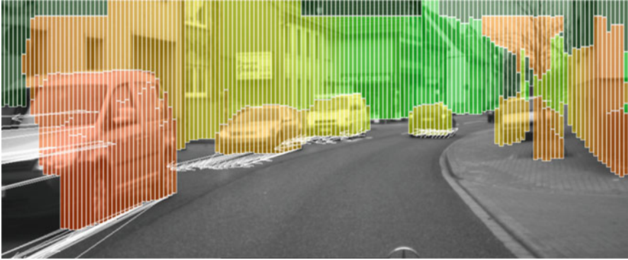
Fig. 15 Representation of the scene from Fig. 5 with Stixels. Distances are color coded; white rectangles define the Stixel outline. The white arrows indicate speed and motion direction
