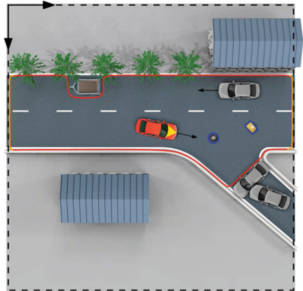
Fig. 8 Parametric Free Space ( PFS ) map in an exemplary driving scenario. The map only represents relevant free space by a closed curve ( red : obstacle boundary, orange : unknown environment boundary) around the ego vehicle and geometric primitives ( blue ) if enough free space has been mapped to drive around the obstacles
