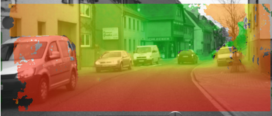
Fig. 5 Color-coded disparity image obtained by SGM ( red nearby . . . green far) overlaid on the original image. A visually error-free disparity image is generated, similar to the GraphCut result
