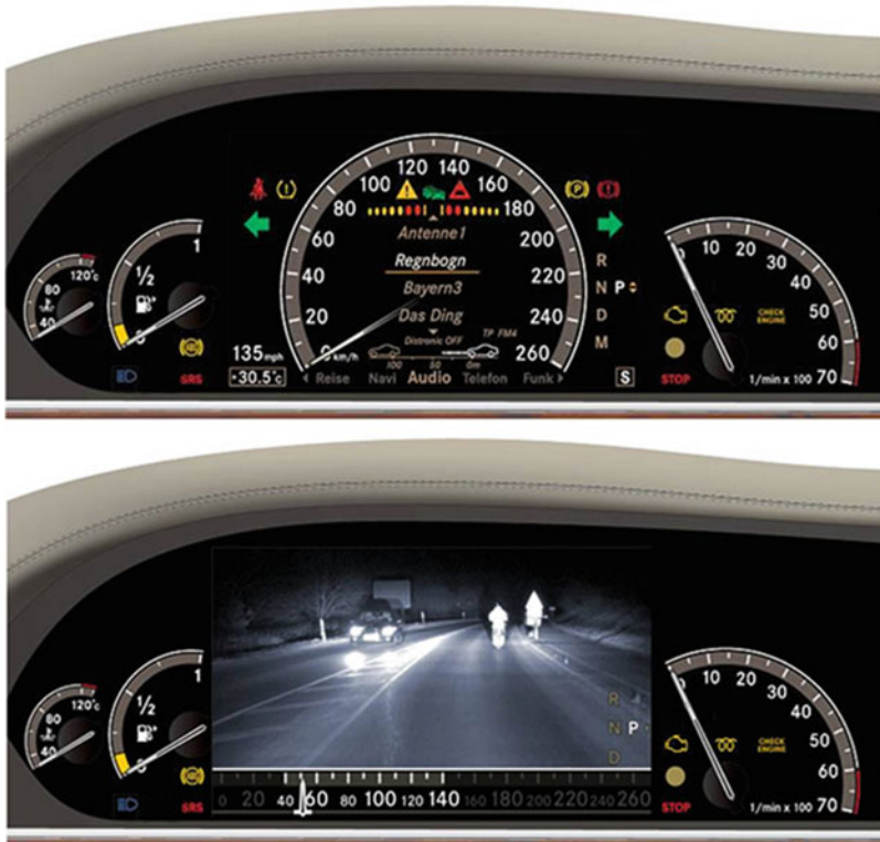
Fig. 5 Instrument cluster with large graphic display (8" diagonal); normal mode ( top ) and in night vision mode ( bottom )
