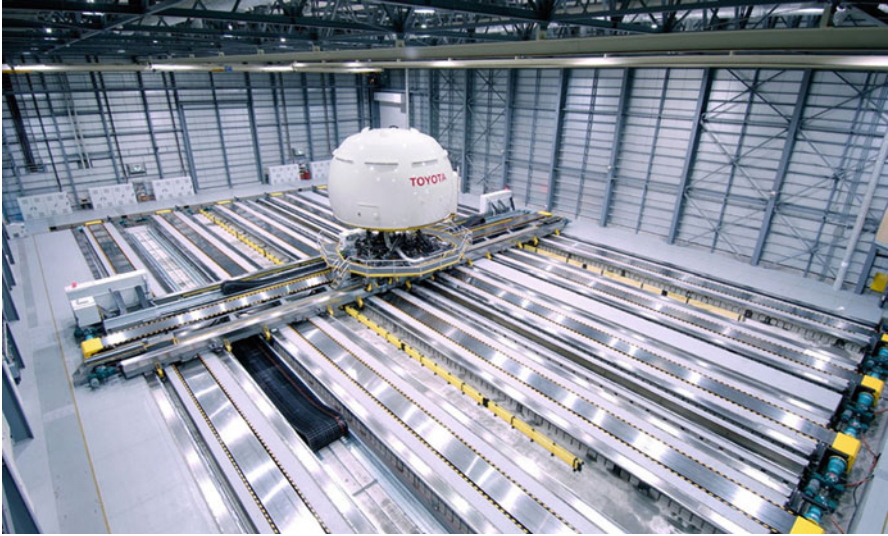
Fig. 2 Toyota's driving simulator in Higashi-Fuji (Murano et al. 2009)
