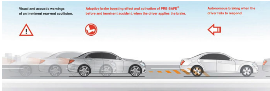
Fig. 1 Driver support by COLLISION PREVENTION ASSIST PLUS to avoid or mitigate rear-end collisions
