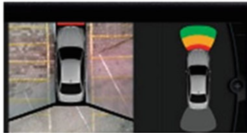
Fig. 7 Examples of viewing systems: side, rear, and top view system
