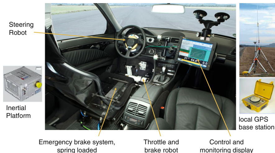
Fig. 2 Robots control throttle, brake, and steering in the vehicle being tested
