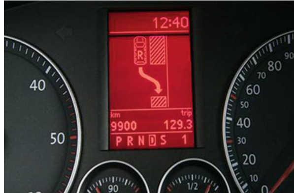
Fig. 4 Graphic module integrated into a mechanical instrument showing the information from a semiautonomous parking system
