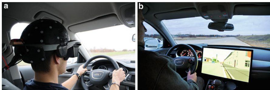
Fig. 2 Potential visualization forms in the VIL: (a) driver with HMD visualization, (b) screen visualization
