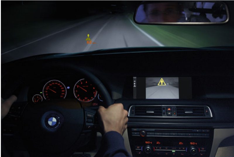
Fig. 9 FIR night vision display with warning from a pedestrian (Photo courtesy of BMW)
