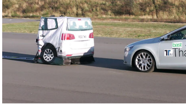
Fig. 2 Euro NCAP vehicle target (EVT) in testing
