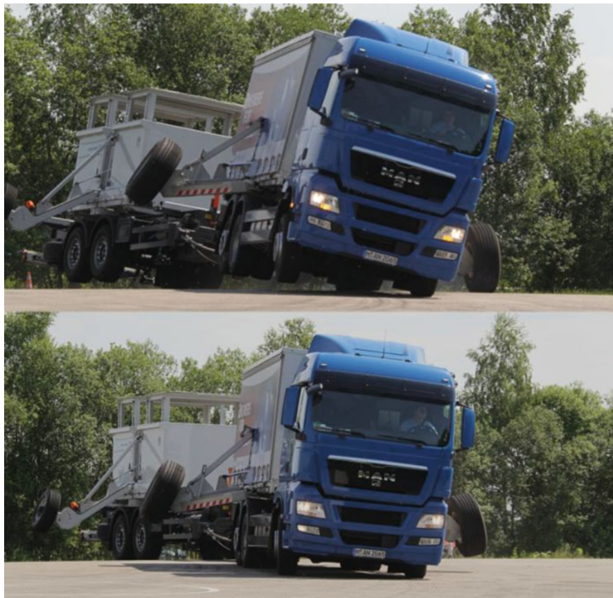
Fig. 8 Cornering at 60 km/h without/with ESP at high friction value with fully loaded semi-trailer combination (Source: Knorr-Bremse)
