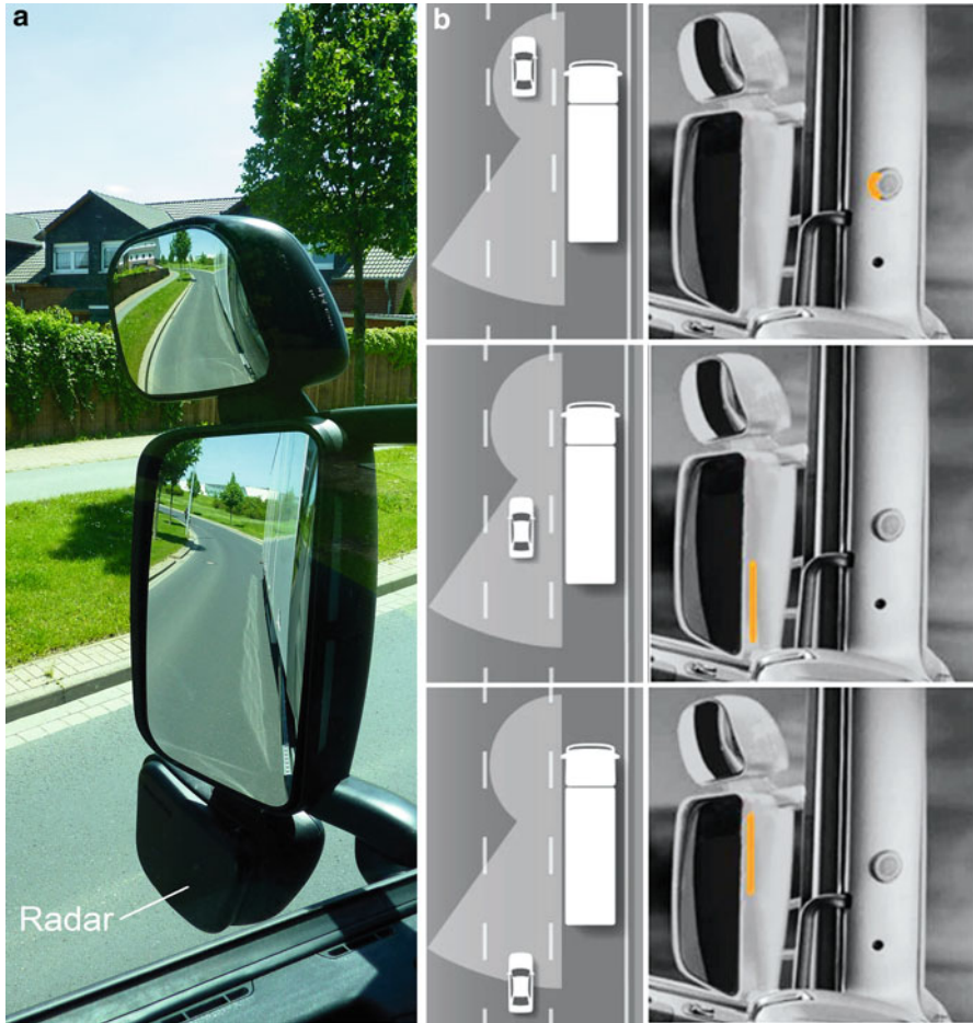
Fig. 9 Prototype from Scania: (a) Mirror with additional RADAR sensor. (b) Zone-based warning system with three LED lights (Degerman et al. 2012)
