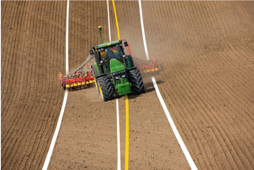
Fig. 13 Tractor on side hill slope with passive implement guidance John Deere iGuide™
