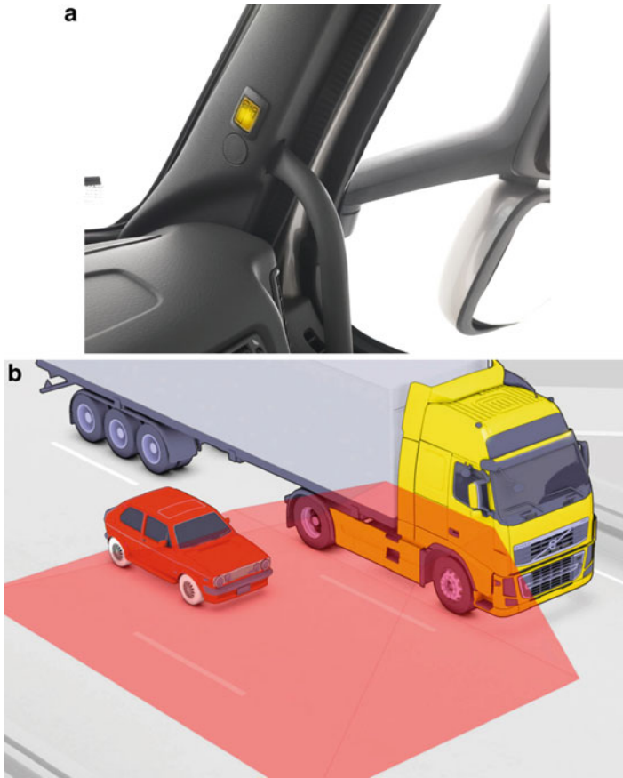
Fig. 8 “Lane Changing Support” from Volvo Trucks (Volvo 2011). (a) LED light on the A-pillar near the grabpole. (b) Monitored area on passenger side
