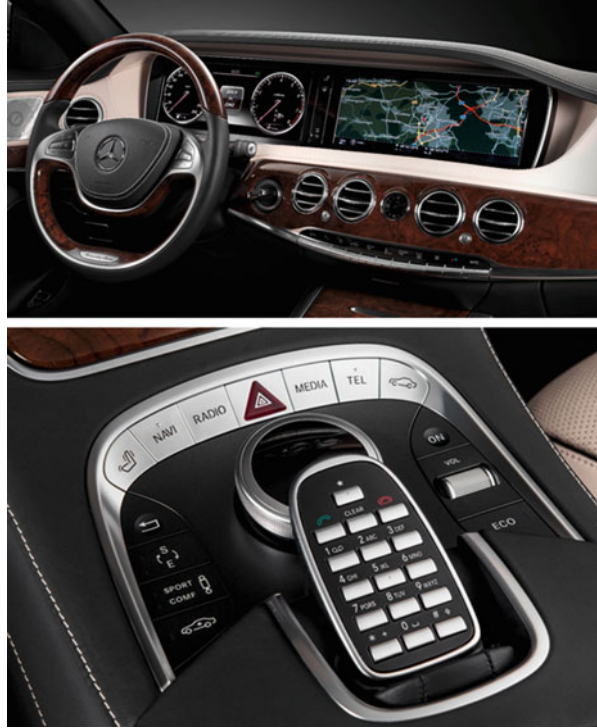
Fig. 6 Dashboard of the Mercedes S-Class 2013 ( top ) and operating element for all driver information functions ( bottom )
