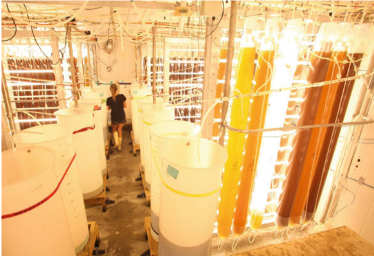
Fig. 6 Microalgae production for aquaculture species feed. The microalgae production facility at the Cawthron Institute in Nelson, New Zealand. Hanging plastic bags are used as photobioreactors for the growth of several monospecies of microalgae, which are used to provide high nutritional quality food for both research use and commercial scale shellfish production. At this facility much of the production is continuous where harvested, algae collects in 200 L white bins ( centre ). Algae from these bins are supplied to juvenile shellfish species, such as oysters and New Zealand Greenshell™ mussel, by a computer-control pneumatic pumping system. Some facilities rely on batch cultures of algae, which are less efficient on an industrial scale. The Cawthron Aquaculture Park also has ~1 ha of outdoor open ponds for mixed-species microalgal production as bulk food for developing shellfish species. Credit Cawthron Institute, Nelson, New Zealand
