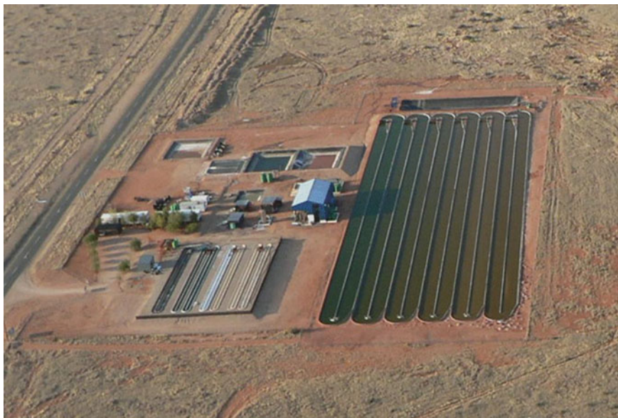
Fig. 3 Aerial view of open raceway ponds used for the production of \beta -carotene near Uppington, South Africa
