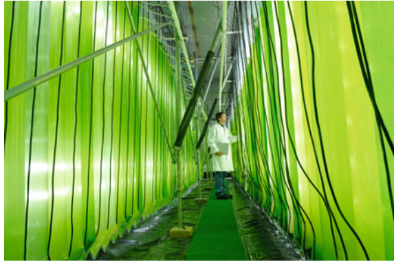
Fig. 5 Semi-continuous bag cultures of microalgae for production of valuable compounds (Image G. Stirling)
