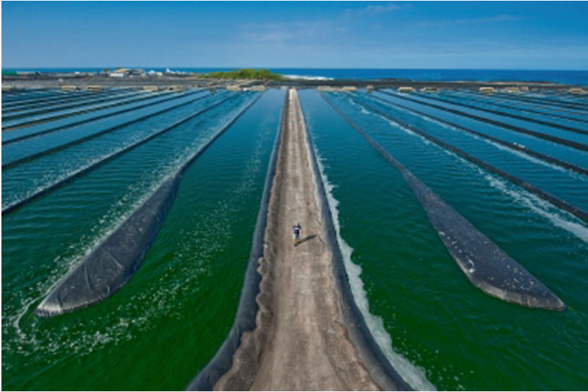
Fig. 2 Raceways ponds for microalgal food production. Raceways are a pond style for suitable for microalgal growth that optimizes light utilization in a given unit area, in a cost-effective manner. Open ponds are managed for continuous production of microalgae. The technology has been developed over the last 40 years resulting in a well-understood industrialized production method for many species. The commodity-scale is demonstrated by the size of the figure walking between raceways in the centre of the image. Credit Cyanotech Corporation, Hawaii, USA
