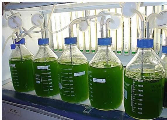
Fig. 6 An early monoseptic stage of production of an algal inoculum for a small raceway
