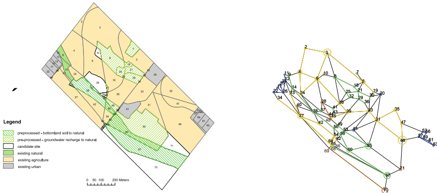
Fig. 1 The preprocessed example data set, primal planar graph (left) and dual graph (right)
