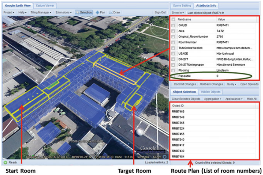
Fig. 11 Route plan for the user from start to target room based on the network model provided by the scenario manager after restricting room no RMB7411 to pass through
