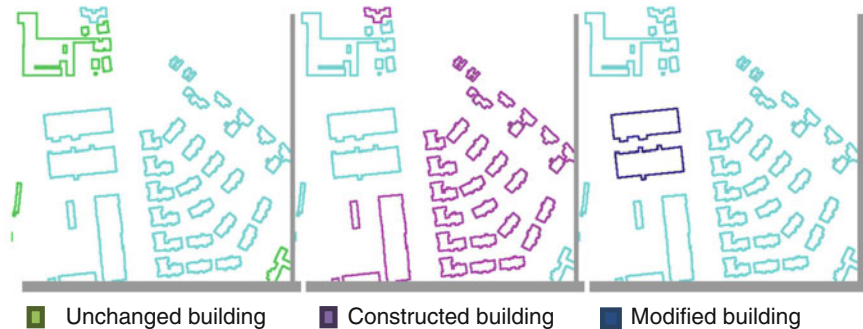
Fig. 12 Comparison on sathonay camp (zoom in on the presented box Fig. 11, right). Left unchanged buildings are in green . Middle created buildings are in purple . Right changed buildings are in dark blue
