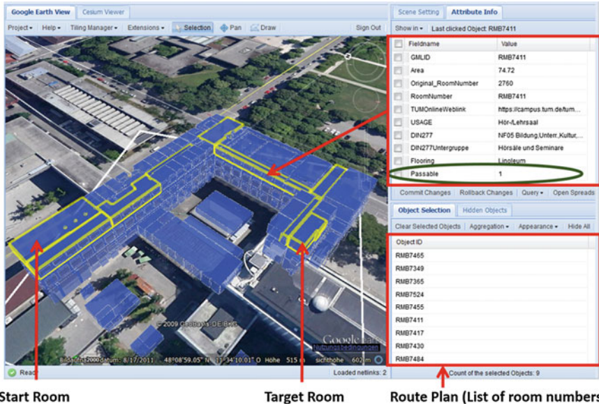
Fig. 10 Route plan with all the semantic and geometric information of the route from the start room to the target room based on the main network model provided by the building administrator
