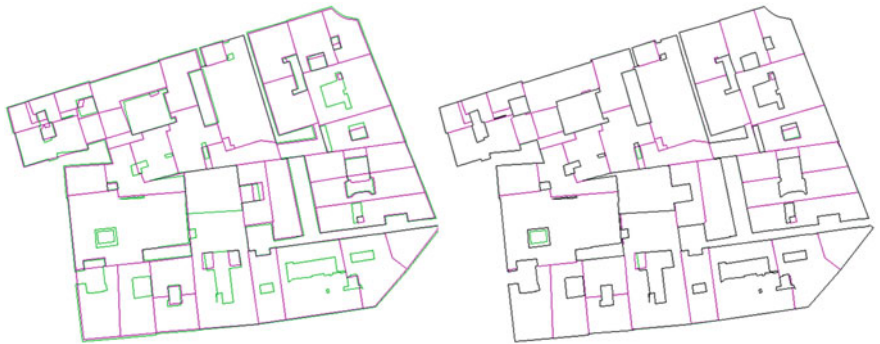
Fig. 17 Cutting according to the cadastre. Left juxtaposition of the cadastre with the CityGML data. Right result cutting
