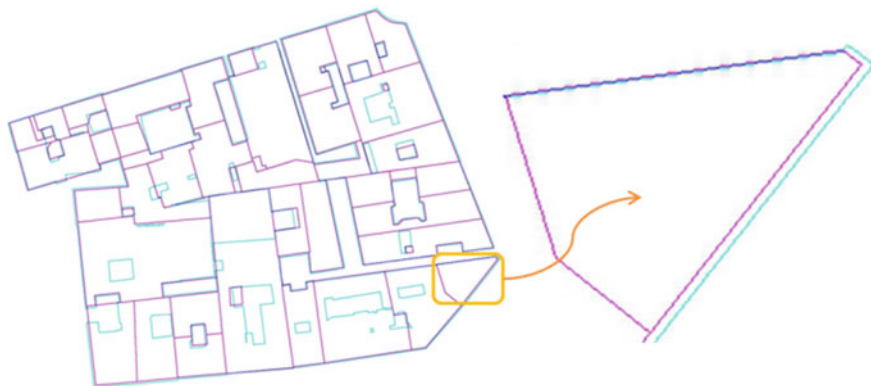
Fig. 9 Difference between a CityGML building ( cyan ) and a cadastral one ( magenta )
