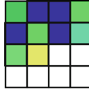
Fig. 4. The payload as 4 by 4 texture padded with 6 words of 0 when interpreted as RGBA pixel format.
