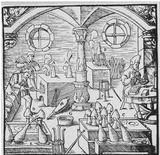
Fig. 2.2 Agricola's illustration of the acid parting of gold and silver [16]. A—Ampullae arranged in the vessels. B—An ampulla standing upright between iron rods. C—Ampullae placed in the sand which is contained in a box, the sprouts of which reach from the opercula into ampullae placed under them. D—Ampullae likewise placed in sand which is contained in a box, of which the sprout from the opercula extends crosswise into ampullae placed under them. E—Other ampullae receiving the distilled aqua and likewise arranged in sand contained in the lower boxes. F—Iron tripod, in which the ampulla is usually placed when there are not many particles of gold to be parted from the silver. G—Vessel
