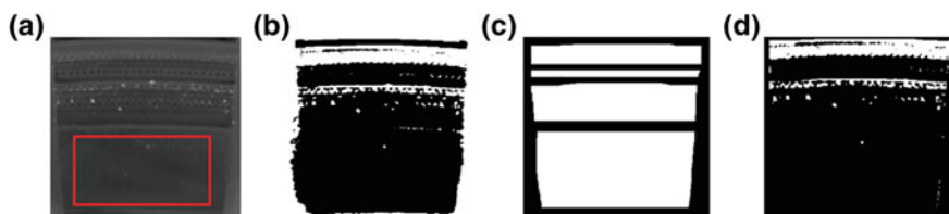
Fig. 8.3 Illustrates the data processing stage of threshold selection area (a), threshold result (b), filtermask (c), and filtered threshold result (d)
