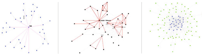
Fig. 2. Figure depicting different types of complex network structures. From left to right: Single Hub , Multiple Hub , Core&Periphery .
