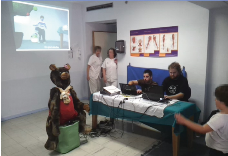
Fig. 3. A snapshot of a rehabilitation session at the Hospital Universitario Virgen del Rocío (Seville). The robot Ursus is a robotic platform with moving head and arms, that makes intensive use of verbal and non-verbal tools to engage the patient in the therapeutic session.
