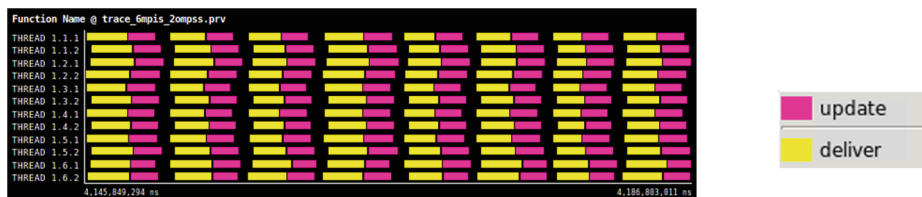
Fig. 12. Task view of some iterations of a hybrid version (6 MPI × 2 OmpSs threads) (Color figure online)
