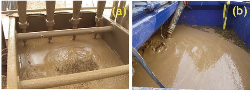
Fig. 10.1 Photographs of (a) water-based mud and (b) oil-based mud. Copyright permission was obtained from Zeal Environmental Ltd. ( http://www.zealenvironmental.com/ )
