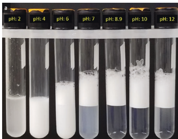
Fig. 8.23 Effect of pH alternation on foam stability of TSP-PO45-COOH surfactant [150]. Permissions related to the material excerpted were obtained from ACS, and further permission should be directed to ACS; Singh, R., Panthi, K., Weerasooriya, U., & Mohanty, K. K. (2018). Multistimuli-Responsive Foams Using an Anionic Surfactant. Langmuir , 34(37), 11010–11020. doi: https://doi.org/10.1021/acs.langmuir.8b01796
