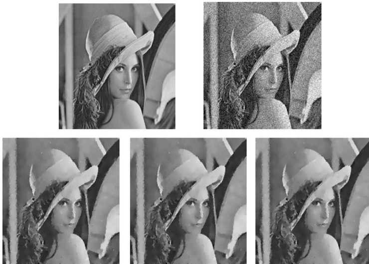
Fig. 1. Lena noise free image (Top Left) , noisy image with sigma= 0.01 (Top Right), restored image using Bazaran model (Down left), SOR solver (middle) and Hybrid BiCGStab solver (Right)
