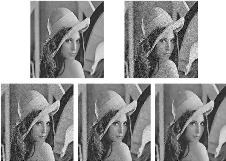
Fig. 3. Lena noise free image (Top Left) , noisy image with \sigma= 0.01 (Top Right), restored image using Bazan model (Down left), SOR solver (middle) and Hybrid BiCGStab solver (Right) for 40 iterations.
