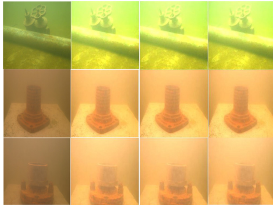
Fig. 1. Result of Image enhancement method: First column: original images, Second column: after homomorphic filtering, Third column: after curvelet denoising, Last column: after LBP- Diffusion
