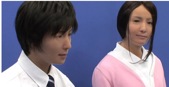
Fig. 1. The Actroid androids in the male (left) and female (right) versions. This experiment used the Actroid-F, the female version of the Actroid robots.
