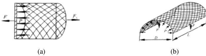
Fig. 8. Force analysis (a) in longitudinal direction, (b) in normal direction
