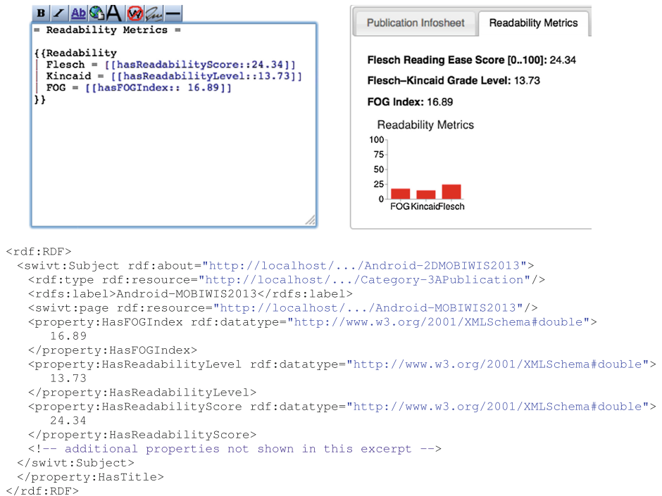
Fig. 3. Wiki template with semantic properties (left), preview in browser (right) and the RDF document (bottom) generated by Semantic MediaWiki
