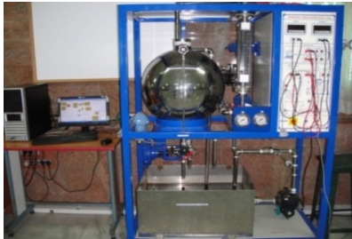
Fig. 1. Experimental setup of spherical tank
