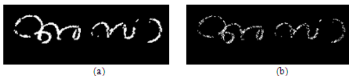
Fig. 2. Illustration of (a) Magnitude, and (b) Direction of the word image shown in Fig.1(a)
