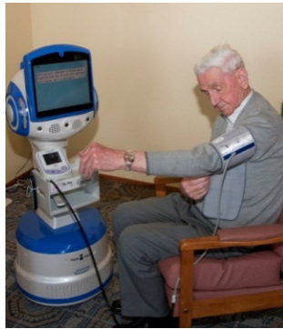
Fig. 1. An older adult measures his blood pressure through our healthcare robot, Charlie, in a rest home. The robot helps older people to measure their vital signs without the aid of caregivers, nurses or family members, and records the data for healthcare providers to check.
