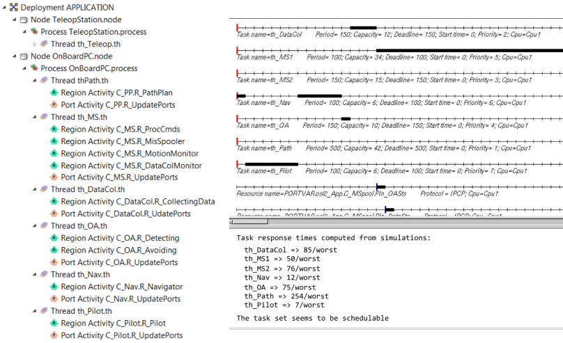
Fig. 6. Deployment model and schedulability analysis with Cheddar
