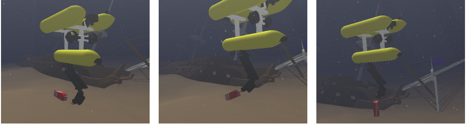
(a) End of approach. The hook is lying on the seabed and the arm cannot follow its setpoint. (b) Lifting. One of the vertical thruster saturates. (c) Recovery complete.
