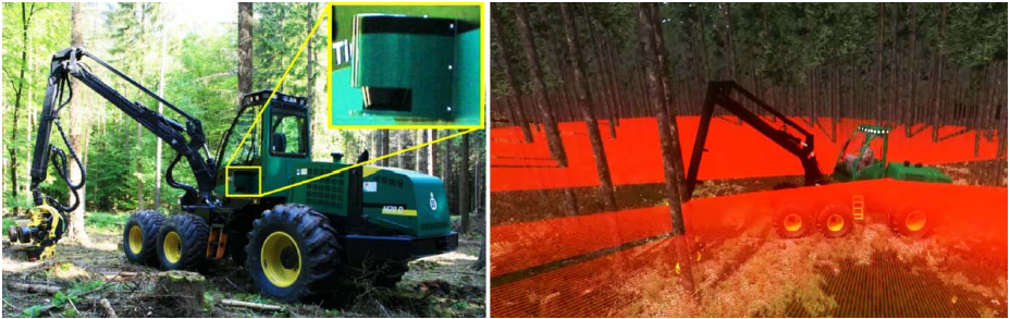
Fig. 9. Real and simulated harvester equipped with 2D laser scanners for forest navigation and harvesting support as an example for knowledge transfer from one project to another
