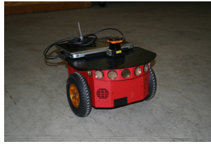
Fig. 1. The P3DX platform equipped with a Hokuyo laser and a laptop for processing
