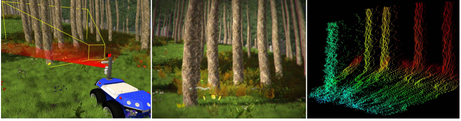
Fig. 1. Simulation of the Seekur Jr mobile robot platform. This Virtual Testbed includes the real-time simulation of the robot itself, as well as several sensors (left: LiDAR sensor; middle: digital camera; right: Time-of-Flight camera) for testing and development of novel navigation approaches.
