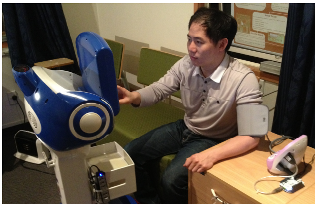
Fig. 1. A human user measures his vital signs using the healthcare sensor managing system with the guidance of a healthcare robot. The measured vital sign data is sent to a medical server via the healthcare robot and caregivers can check the health condition by observing the data.
