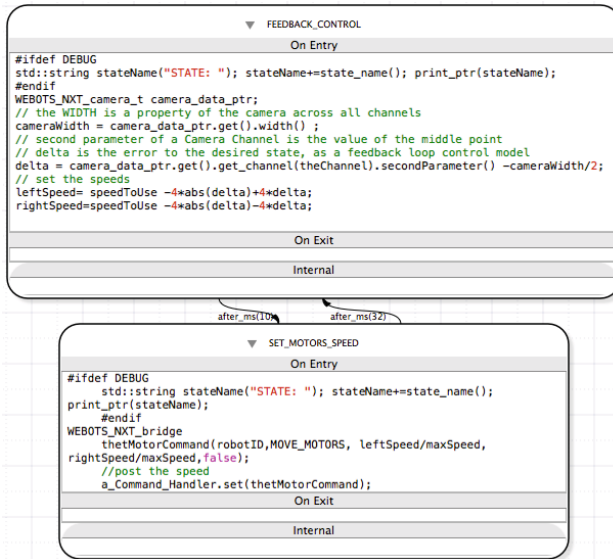
Fig. 3. Two states that use gusimplewhiteboard services to perform a feedback loop to control an ePuck that follows coloured lines
