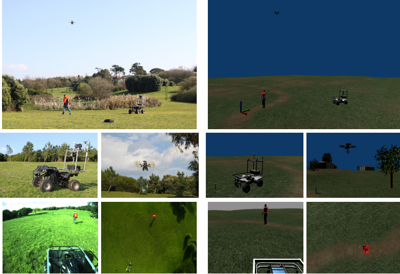
Fig. 2. Top-Left: Experimental scenario[19]. Right: MORSE outdoor simulation environment. Middle - Left: UGV TIGRE[17] and MAV Asctec Pelican. Right: Simulated robots: MAV and the UGV TIGRE developed based on the TIGRE 3D model. Bottom - Left: TIGRE and MAV camera view. Right: Simulated TIGRE and MAV camera view.
