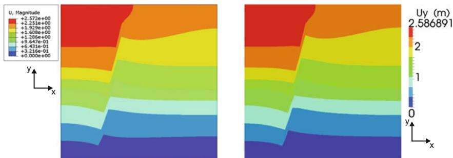
Fig. 10.5 Displacement in the y direction (m) calculated with ABAQUS (left) and OGS (right)
