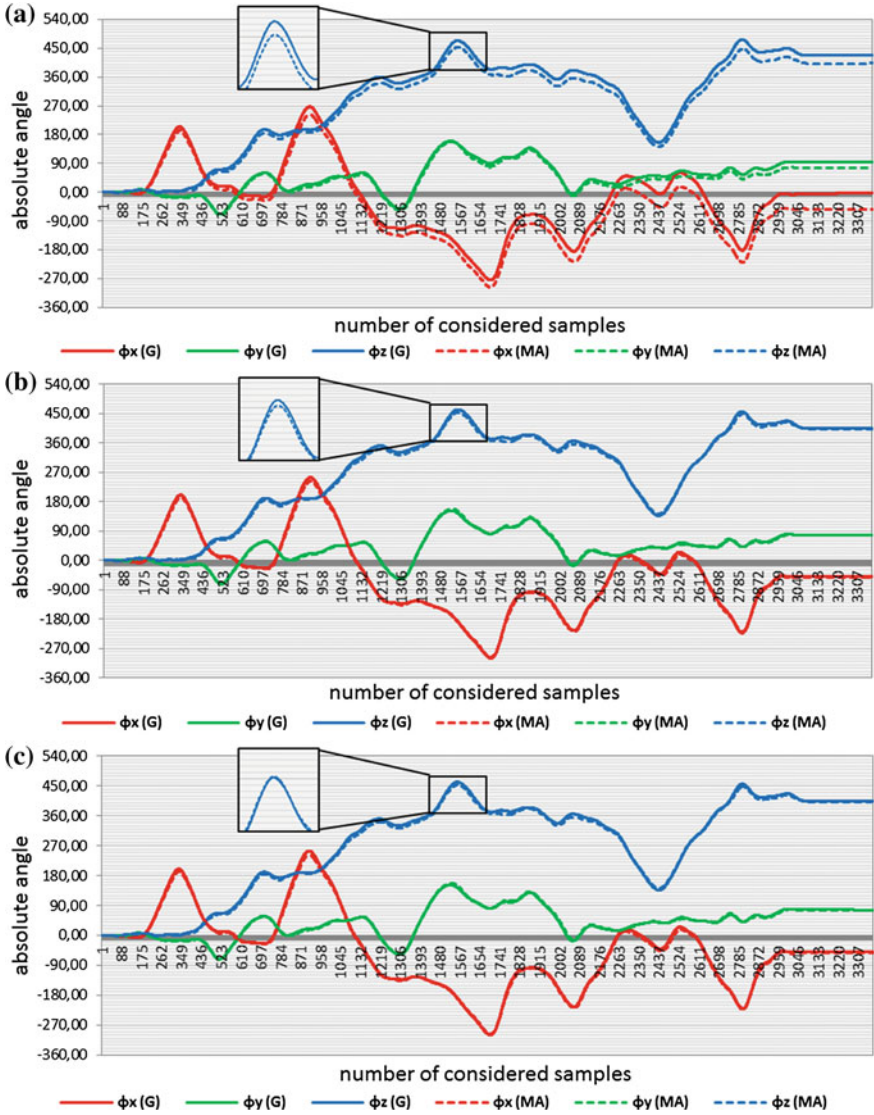
Fig. 8 Reduction of the uncertainty parameters of the gyroscope by the comparison of the data of the gyroscope and the accelerometer plus magnetic field sensor (MA): a uncalibrated data, b drift corrected data and c drift corrected and calibrated data
