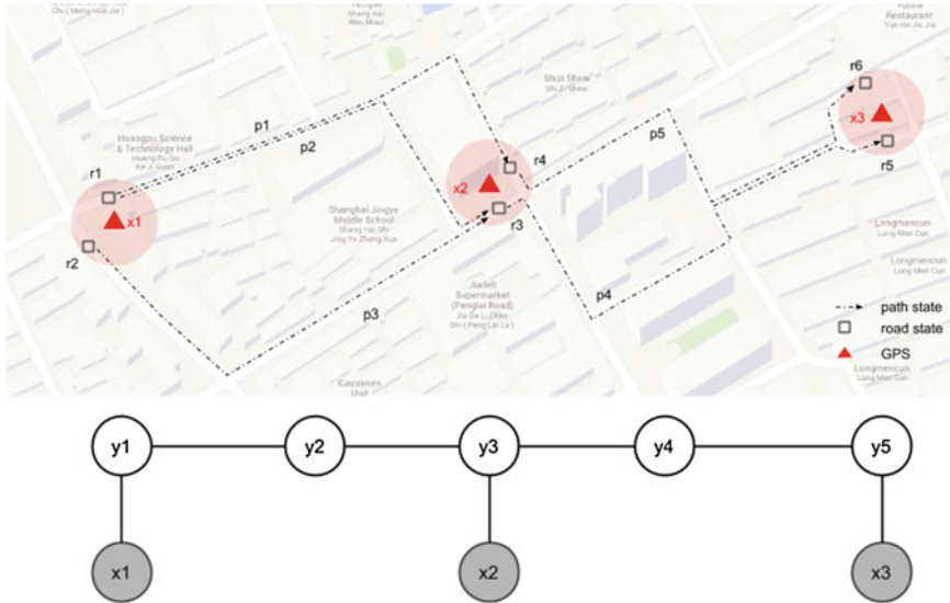
Fig. 2 A chain-structured CRFs for 3 GPS observations. The map on top illustrates the simplified situation of identifying road states and path states given GPS observations in the road network. This requires 5 random variables, y_1 : \{r_1, r_2\} , y_2 : \{p_1, p_2, p_3\} , y_3 : \{r_3, r_4\} , y_4 : \{p_4, p_5\} , y_5 : \{r_5, r_6\} , to build the CRFs for map matching. Thus, nodes y_1, y_3, y_5 linking with observations (black circles) are point nodes while nodes y_2, y_4 are path nodes
