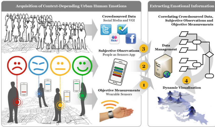
Fig. 1 Urban emotions concept: (1) emotion sensing, (2) ground-truthing using people as sensors, (3) extraction of emotion information from VGI, (4) correlating measured and extracted emotions; plus visualisation and enrichment of urban planning processes
