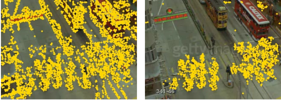
Fig. 2. Interaction flow. The extracted corner features (left column); the same frame with the interaction flow overlaid (right column).
