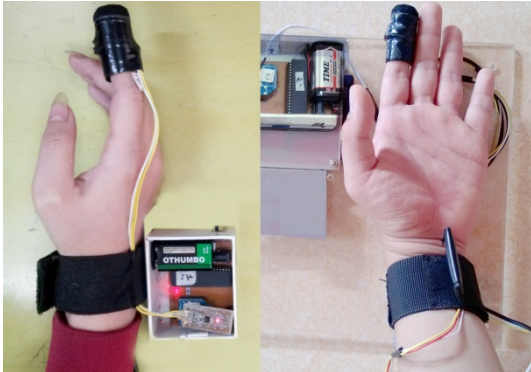
Fig. 9 The base node is in charge of collecting data from the sensor nodes of each patient
