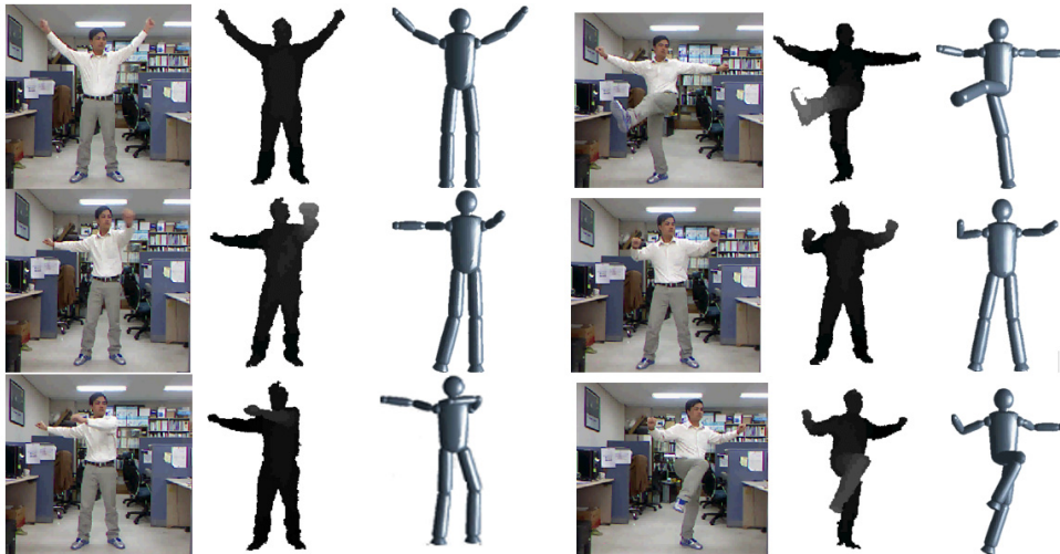
Fig. 6 Sample illustrations of our proposed 3-D human pose recovery method on depth images with the occlusion of arm or leg body parts
