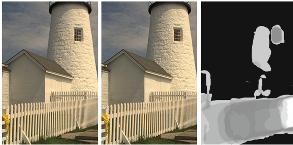
Fig. 4. From left: an example reference image, the same image but with artefacts caused by the GBI demosaicing technique (see the Moire artefacts on the fence), a map of Kendall coefficients (brighter pixels denote higher agreement between observers)
