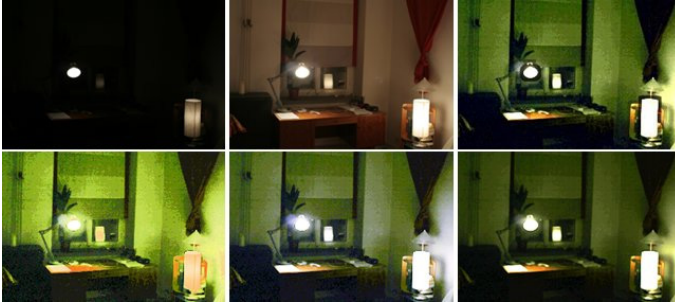
Fig. 4. Office very dark dataset: (Top left) Original Image, (Top middle) Reference Image, (Top right) Dong's method, (Bottom left) HE, (Bottom middle) CEM, (Bottom right) Proposed method
