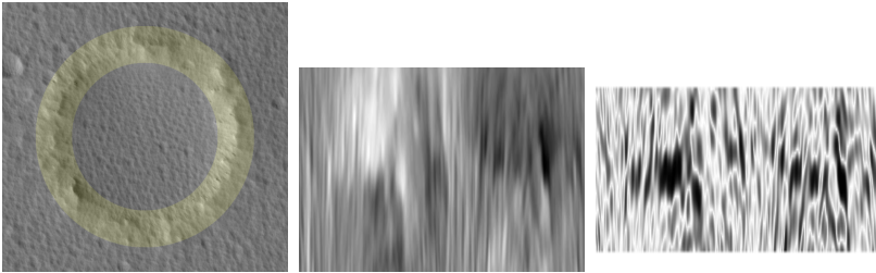
Fig. 1. Image transformation: original image and sampling points (left), polar image (centre) and edge map (right)
