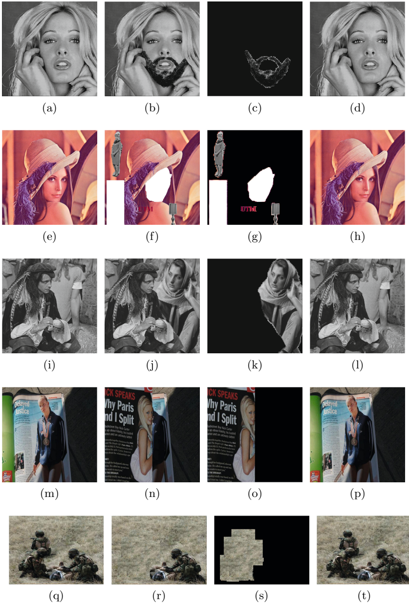
Fig. 2. Malicious Tampering Attacks. (a) Watermarked Blond ,(b) General tampering, (c) Tampered located, (d) Recovered image (PSNR= 38.42 dB), (e) Watermarked Color Lena(PSNR= 43.87 dB), (f) Multi Tampering , (g), Tampered located, (h) Recovered image (PSNR= 34.22 dB),(i) watermarked pirate, (j) Collage attack , (k) Attack detected ,(l) Recovered image (PSNR= 33.44 dB),(m) Watermarked magazine, (n) Collage attack 50 % , (o) 50 % CA attack detected ,(p) Recovered image ,(q) Watermarked soldiers, (r) CAA and VQ attack , (s) Attack detected ,(t) Recovered image
