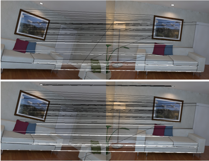
Fig. 1. Matching with FAST-BRIEF combination (top) and tracking (bottom). Matches with reprojection error less than 2 are marked white.
