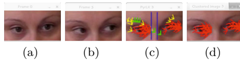
Fig. 5. Sample optical flow images. Optical flow is calculated between (a) and (b). Optical flow results in (c): green vectors for the softer movements, yellow for intermediate and red for strongest movements. Stronger vectors in (d) after filtering the rest.
