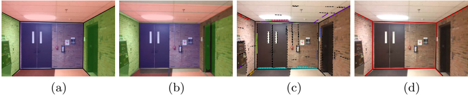
Fig. 3. Layout and correspondent plane orientation, (a), and the orientation map computed from the observed lines, (b). Both orientations maps are compared to compute S_{omap} . Lines supporting the model, S_{lines} , (c), and evaluated hypothesis (black) and closest observed layout (red), used to compute S_{model} , (d). Best seen in color.
