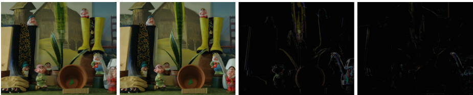
Fig. 7. Comparison of dense and sparse image interpolation on the Middlebury “Dwarves” dataset [18]. Left: Dense, TV-L1 flow, e_{RMSE} = 11.19 , Sect. 2.2. Right: Sparse, guided matching, e_{RMSE} = 6.08 , Sect. 2.1. The left two images show interpolations for one skipped frame, which we take as ground truth. The right two images show difference images of the algorithms’ results and the ground truth. Despite the large camera motion, our sparse approach still manages to establish reliable correspondences.
