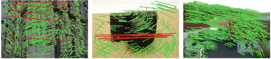
(a) Playground Filter. Matches are globally filtered using clustering. Note, that no outliers are detected in the right most example, as the relative difference between large and extreme displacements is not significant enough.
