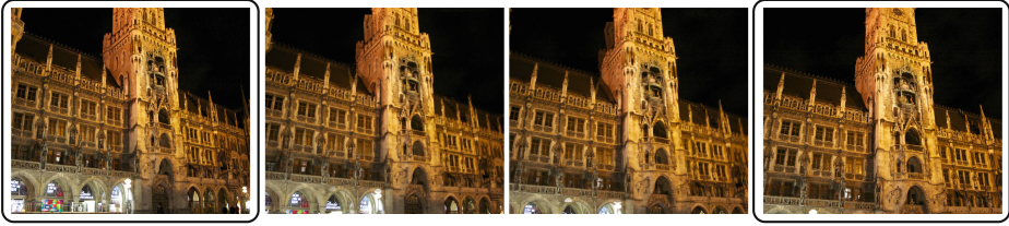
Fig. 1. Spatial view point interpolation between two images. Our approach robustly handles wide-baseline view point interpolations. From left to right: source image, interpolation at t = 1/3 , interpolation t = 2/3 , target image.
