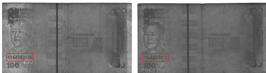
Fig. 1. RMB images scanned by contact image sensor
