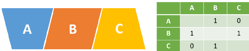
Fig. 10. Illustration of neighbor check and adjacency matrix
