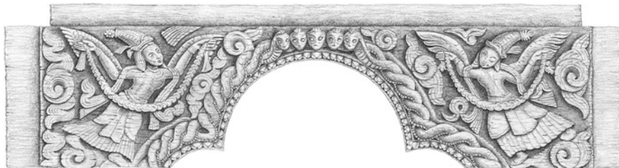
Fig. 10 Bhaktapur, Kuthumaṭh, uppermost panel of the trefoil central window (24.2 × 91.6 cm) of the eastern wing of the courtyard, established in 1749. The relief carving is 3 cm deep, while the fivefold snake hood has been added to the panel and projects 3 cm outward. A pair of garland bearers graces the opening, their arms fully stretched outwards and equipped with wings, which originate from their shoulders. Their outlandish tapering headgear, crowned by flowers, demonstrates the introduction of new conventions, further supported by their open, long-sleeved shirts, and long, frilled gowns, which extend to their ankles. The fluttering scarves faintly recall the ancient outfits worn by wisdom bearers. Slight variations suggest that a couple is depicted: the figure on the left could be female, as evidenced by long hair, a necklace and a long garland of pearls. The figures are framed by scrolled cloud motifs of the Chinese fashion. The opening is framed by pairs of twisted snake bodies, with a fifth head marking the centre. Drawing by Axel Weller, 2009
