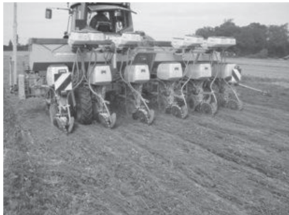
Fig. 21.3 Direct sowing of maize on a rolled alfalfa cover crop at site A (France). (Source J. Peigné—ISARA Lyon)
