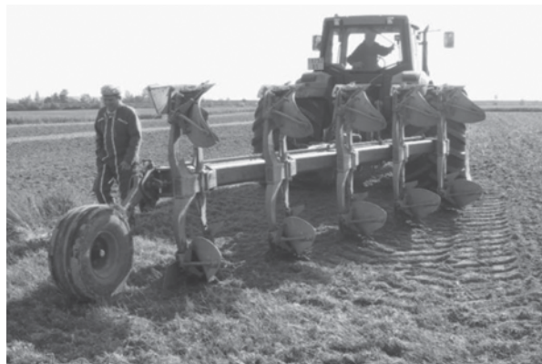
Fig. 21.10 Shallow plough tested in at site A (France)—the plough is adapted to work at 18 cm depth, on-land and without skim coulters
