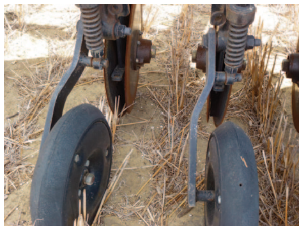
Fig. 14.2 Disc seeders cause minimal soil disturbance and can cope with large residue loads
