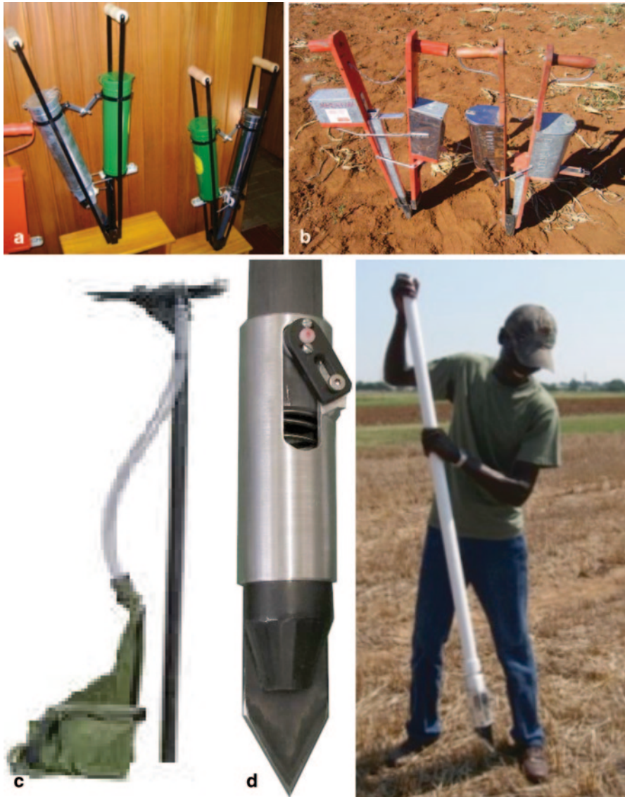
Fig. 5.7 Jab planters. (a) cylindrical metallic twin hopper; (b) rectangular metallic twin-hopper jabs; (c) Li seeder and (d) dibbler. (1) Soil- and residue-cutting device; (2) furrow-opening device; (3) fertilizer- and seed-covering device (4) seed-firming device
