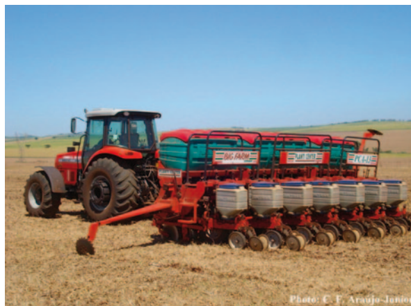
Fig. 16.4 Big farm seeder for direct seeding in crop residues. Floresta, State of Paraná, Brazil
