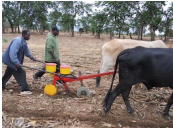
Fig. 18.4 Seeding through a mulch of crop residues with a direct seeder and fertilizer distributor
