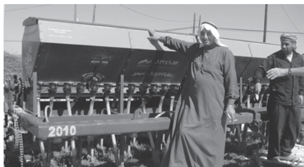
Fig. 9.4 Syrian farmer, Ismail Jarrad, purchased an Ashbal zeo tillage (ZT) seeder made by Ibrahim Shibley at Qabbaseen, Syria, in 2011. (Photo: A. Haddad)
