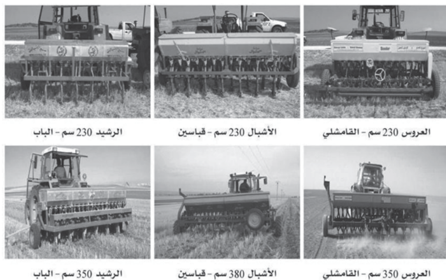
Fig. 9.5 Six of the simple zero tillage (ZT) seeders produced commercially by local village workshops in Syria in 2011. Prices varied from US$ 2000 to 7,000. (Photos: A. Haddad)
