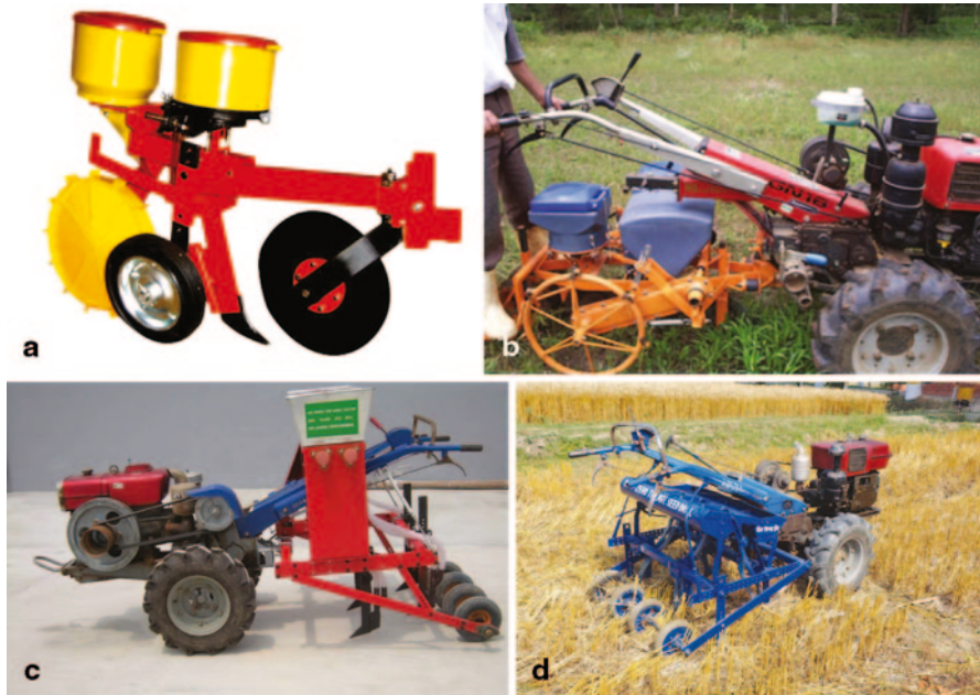
Fig. 5.10 2WT direct CA seeders. (a) Fitarelli; (b) Knapik; (c) ARC Gongli; (d) Bangladesh. 2WT two-wheel tractor; CA conservation agriculture
