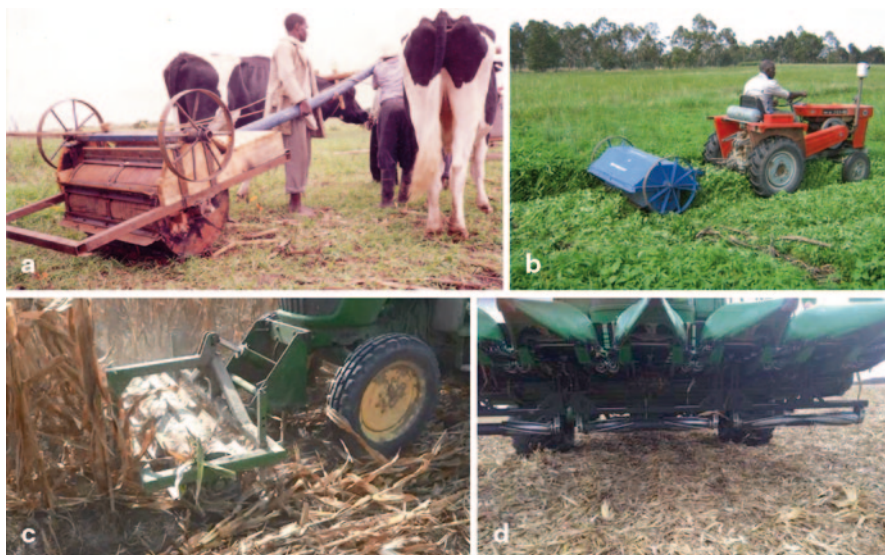
Fig. 5.5 a Knife roller from wood roller; b metallic roller—pulled by small tractor; c tractor knife roller; d stalk roller crusher (attachment to combine harvester)
