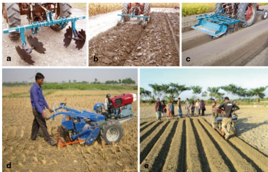
Fig. 5.3 a, b, c Buckeye Tractors' disc bedder and shaper pan for making permanent broad beds. d, e—VMP. VMP versatile multi-crop planter
