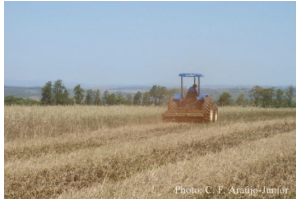
Fig. 16.3 Knife roller used on a black oat cover crop before the cash crop is seeded. Agronomic Institute of Paraná (IAPAR), Londrina, State of Paraná, Brazil
