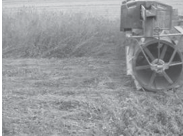
Fig. 21.2 Home-made roller-crimper used at site A (France): steel bars were welded to a roll. The aim of the roller-crimper is to roll over and damage the cover crop before sowing the cash crop. (Source J. Peigné—ISARA Lyon)
