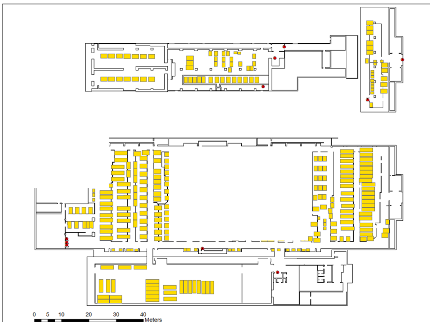
Fig. 1. Indoor space layout of the semiconductor production which is subject of this paper. Yellow rectangles represent devices in the clean room, and red dots represent transfer nodes. The white spaces are intentionally to disguise the complete production layout.
