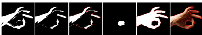
Fig. 5. The process of hands video processing: a) picture with the border; b) the biggest continuous binary object; c) reconstruction of the whole binary object; d) area inside the palm; e) finding control points by the model; f) reconstructed hand's form
