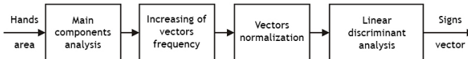
Fig. 4. Functional scheme of pixel visual signs calculation method for the sequence of video frames
