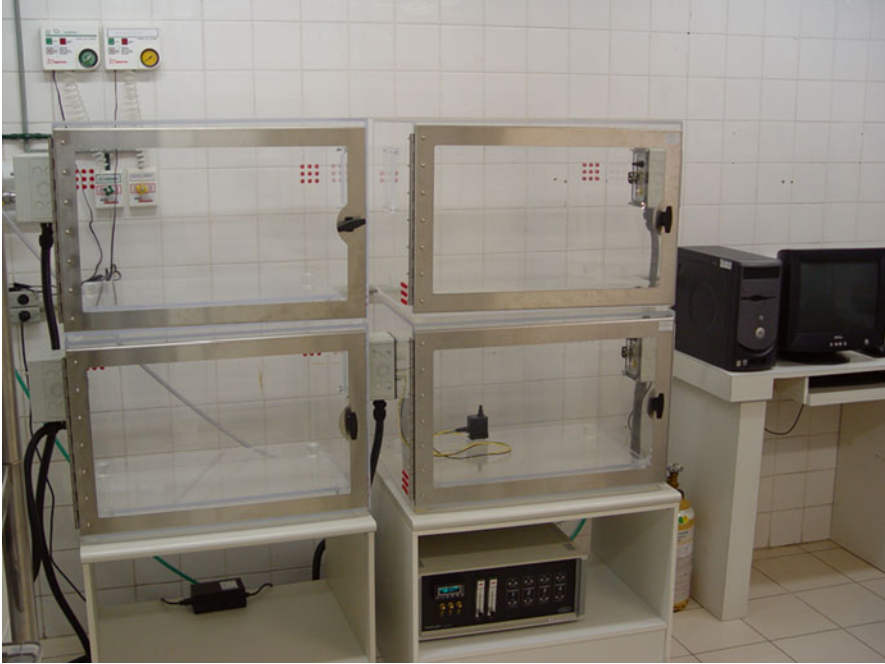
Fig. 24.5 Hypoxia chamber. Intermittent hypoxia is induced in a specially built chamber (30×20×20 in., Oxycycler model A44X0, Biospherix, Redfield, NY, USA) connected to a supply of O 2 and N 2 gas. Sensors measured O 2 concentration, CO 2 concentration (<0.01 %), humidity (40–50 %) and temperature (22–24 °C). Inflow of O 2 and N 2 into the chamber are controlled by a computer programmed to produce cycles of minutes room air to seconds 2–10 % O 2
