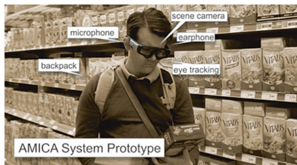
Fig. 11.1 The AMICA system prototype is based on standard technologies, such as a laptop ( backpack ), microphones, earphones, a scene camera and a binocular eye-tracking system
