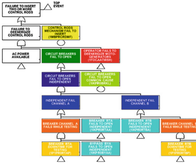
Fig. 28.3 Fault tree for RPS failure
