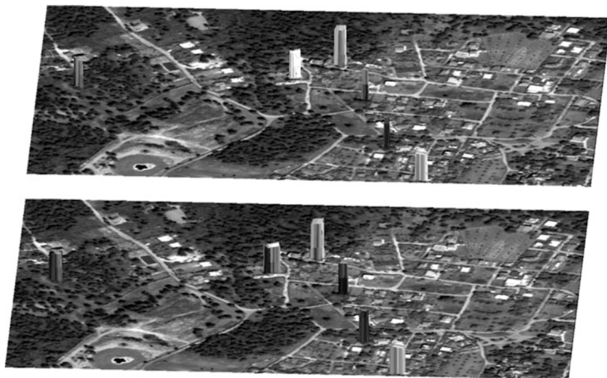
Fig. 10.4 The detected changes (new buildings) in 3D after the application of the unsupervised change detection procedure on QuickBird 2007 and 2009 satellite data. The detected new building in 3D are shown in the upper part, while the 3D buildings from the ground truth data are shown in the bottom . After a close inspection one can observe the low completeness and high correctness detection rates of the unsupervised change detection algorithm
