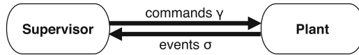
Fig. 5 The basic structure of supervisory control, where one DES (supervisor) commands another DES (plant)
