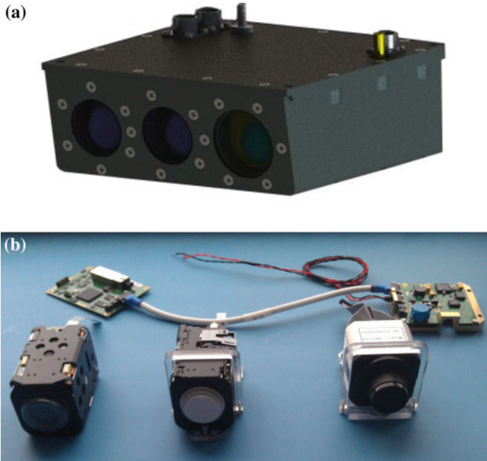
Fig. 8.11 Multi-spectral optical-electronic system: a model of the ESVS optical unit, b the ESVS sensors
