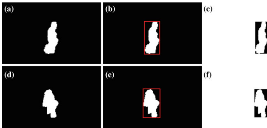
Fig. 2.7 Cropping bounding box process for bending and jumping forward actions in Weizmann dataset: a, c original ASI images for two actions, respectively, b, d bounding box (in red color) for their silhouettes in ASI images, e, f cropped (separated) bounding box regions
