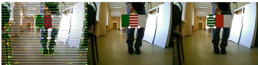
Fig. 5.4 Results of frame processing, when the STG is put on the grayscale component, and two selected rectangles
