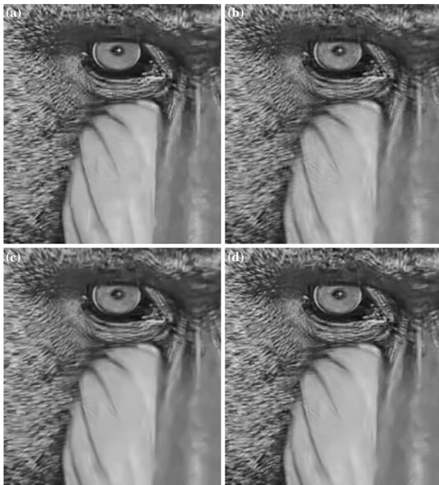
Fig. 10.4 Fragments of AWGN-affected “Baboon” ( \sigma = 25 ) test image reconstruction results (in brackets PSNR, dB and MSSIM): a block matching and 3D filtering (BM3D) [18] (25.46 dB, 0.745), b modification of PCA-based filtering (25.52 dB, 0.748), c sequential scheme (24.90 dB, 0.714), d parallel scheme ( 25.57 dB, 0.750 )
