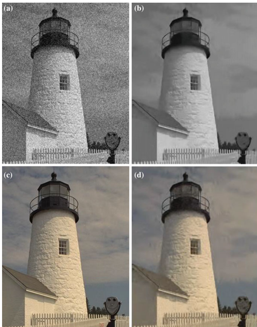
Fig. 10.9 Fragments of test image “Lighthouse” (in brackets PSNR, dB and MSSIM): a noised “raw” image (20.25 dB, 0.422), b non-local PCA (29.98 dB; 0.905), c non-noised true color image ( \infty dB, 1), d non-local PCA + demosaicking (R: 29.63 dB, 0.865; G: 29.91 dB, 0.868; B: 29.10 dB, 0.857)
