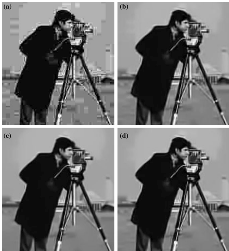
Fig. 10.7 Fragments of JPEG-compressed “Cameraman” ( Q = 6 ) test image reconstruction results (in brackets PSNR, dB and MSSIM): a image compressed with JPEG (25.03 dB, 0.756), b modification of PCA-based filtering (25.79 dB, 0.783), c sequential scheme (25.76 dB, 0.782), d parallel scheme ( 25.92 dB, 0.788 )
