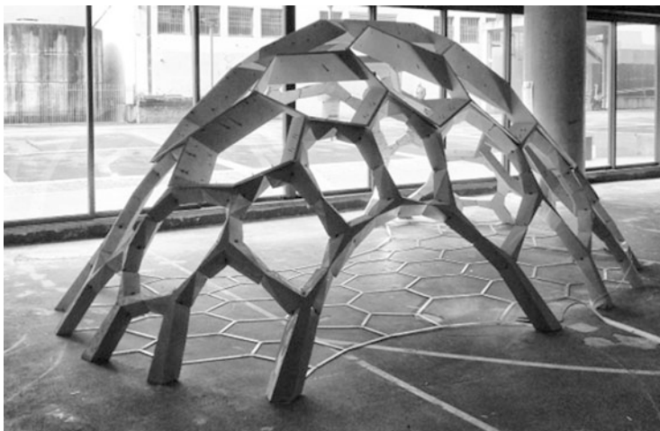
Fig. 1 Form-found structure comprising unique precast concrete elements (Design Experiment 3)
