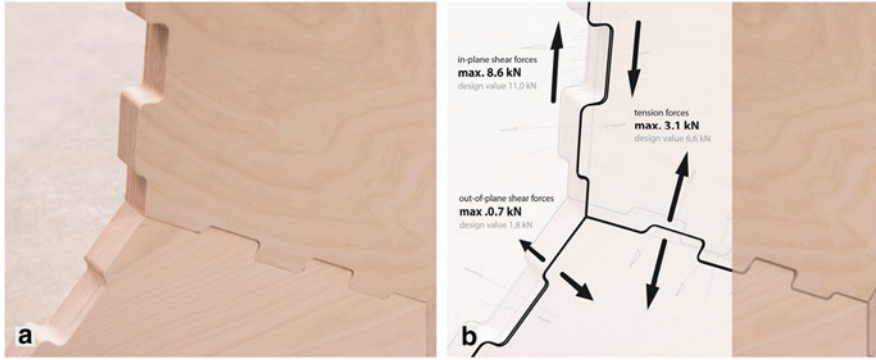
Fig. 5 Visualization of the forces inside the plate structure. The dominant in-plane shear forces are transferred through the plate’s finger joints
