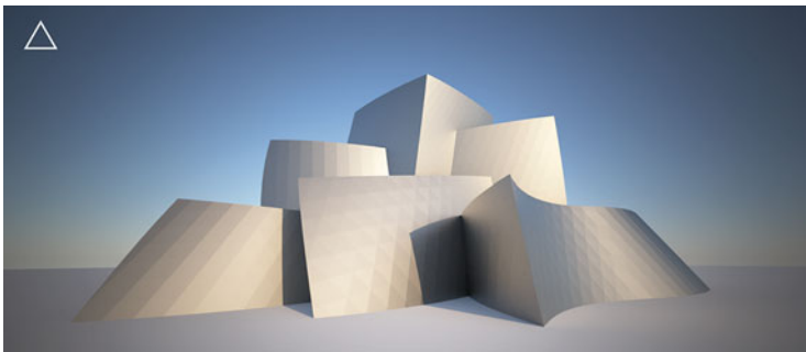
Fig. 5 Architectural design with large scale developable patches that are realized entirely by repeating a single, planar, equilateral triangle
