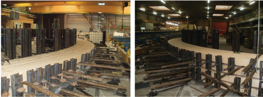
Fig. 6 Photos showing the bending process of the glulam timber
