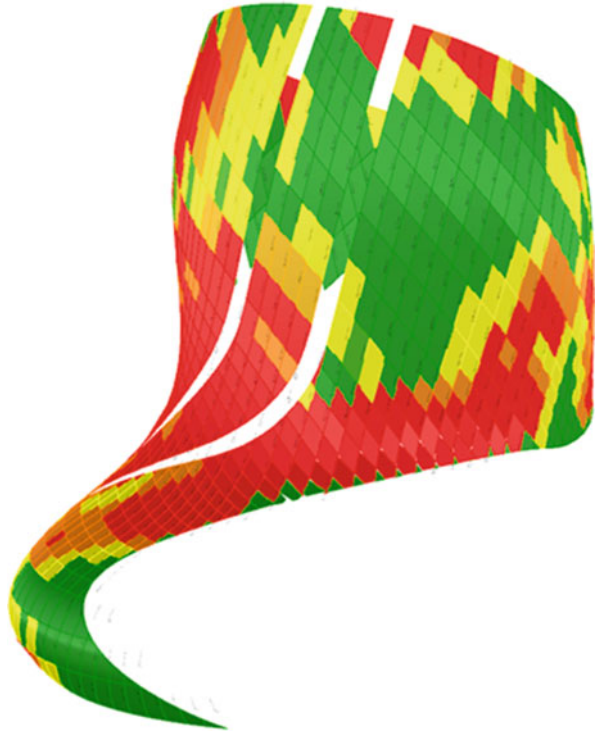
Fig. 12 Results mapping: green: 0–10 mm, yellow: 10–20 mm, orange: 20–30 mm, red: over 30 mm
