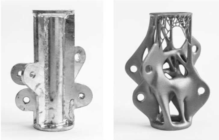
Fig. 11 A model of the traditional node, scaled to 40 %, in galvanized steel. It is produced in the traditional way by cutting and welding ( left ). A model of the node, scaled to 40 %, produced by Additive Manufacturing in Maraging steel ( right )
