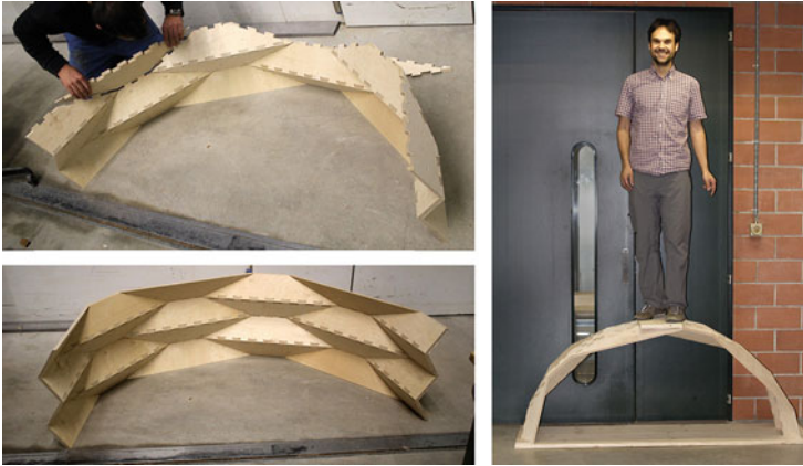
Fig. 8 Folded-plate arch prototype built from 12 mm birch plywood (9-layer, I-I-I-I-I). Assembled without adhesive bonding or metal fasteners. Span 1.65 m, self-weight 9.8 kg
