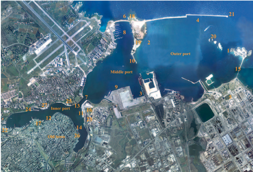
Fig. 24.2 Morphology of the port of Brindisi: Pedagne islands (1), Sant’Andrea island (2), Costa Morena pier (3), Punta Riso dam (4), Petrochemical pole (5), Bocche di Puglia dam (6), Pigionati canal (7), Touristic harbor (8), Passengers and cruise harbor (9), Sea Fort pier (10), Sant’Apollinaire dock (11), Sciabiche dock (12), Carbonifera dock (13), Customhouse dock (14), Capo Bianco dam (15), Punta delle Terrare (16), Swabia Castle (17), Aragonese Castle (18), Sea fort (19), Pedagne lighthouse (20), Punta Riso lighthouse (21), Arsenal (22), Montecatini warehouse (23), Naval boarding school (24), Monument to the sailor (25), Maritime station (26), Naval League and harbor (27)
