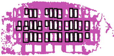
(a) Windows detected in the wall layer.
