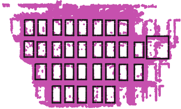
(a) Windows detected in the wall layer.
