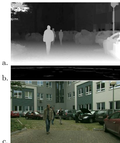
Fig. 1. a. Depth map and b. 2D histogram associated with c. a frame 282 from Poznan Car Park sequence
